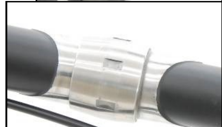
Look at the extreme high quality of the machining of the S&S couplings.
