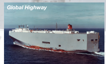
The world’s largest PCC at the time Completed in 1982, 6,300 car capacity
