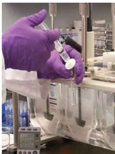
Figure 2. Filtration of the dissolution sample.
