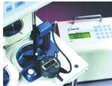
Figure 3. Checking physical parameters prior to the dissolution test.
