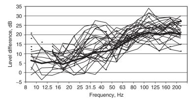
Figure 2. Results of all measurements of level difference and the selected 'level difference curve' that is exceeded by 67% of the measurements.
