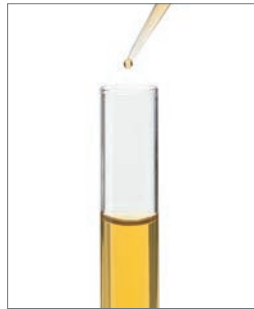
The drop on the tip needs to be removed.
