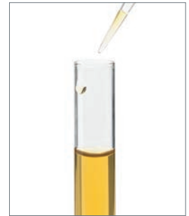
Ensure that you have the proper volume of sample in the tip.
