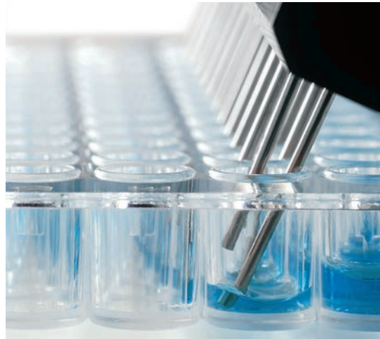
Proper position of manual washer needles for aspirating liquid
