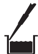
Proper position to dispense reagents into wells containing liquid using a multichannel pipette; above the liquid
