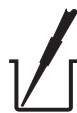
Proper position to dispense reagents into empty wells using a multichannel pipette; in the lower corner of each well
