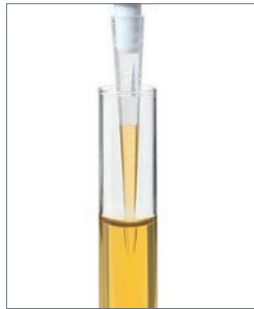
Draw up the calibrated volume of sample into the tip.
