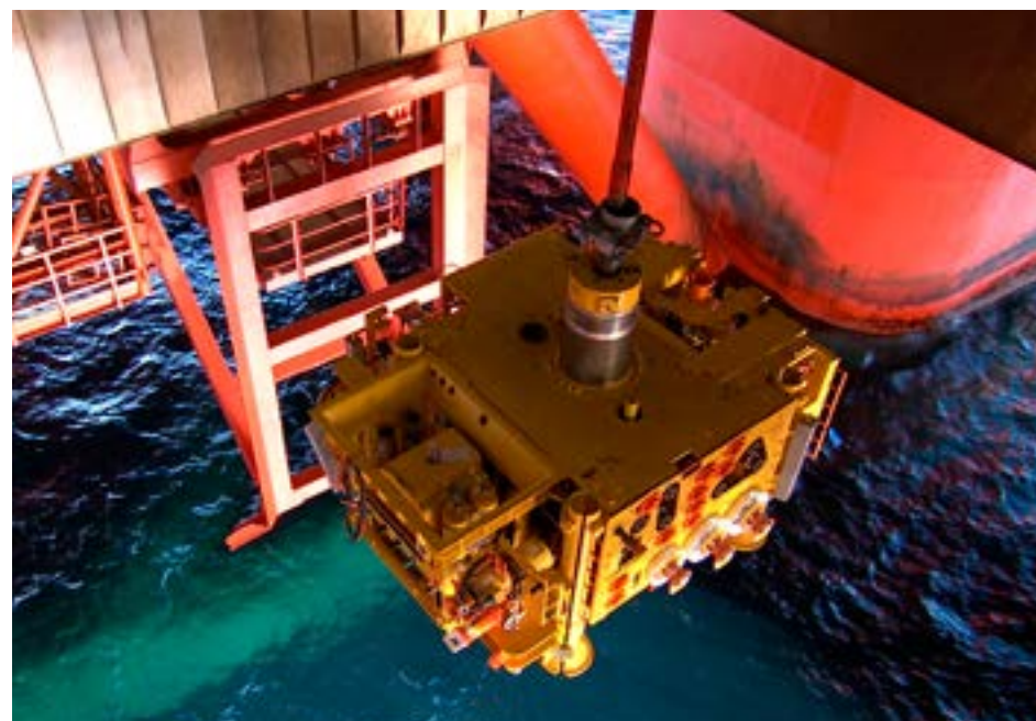
Installation of a Horizontal Xmas Tree (HXT) at the Jette field, from the Transocean Barents.
