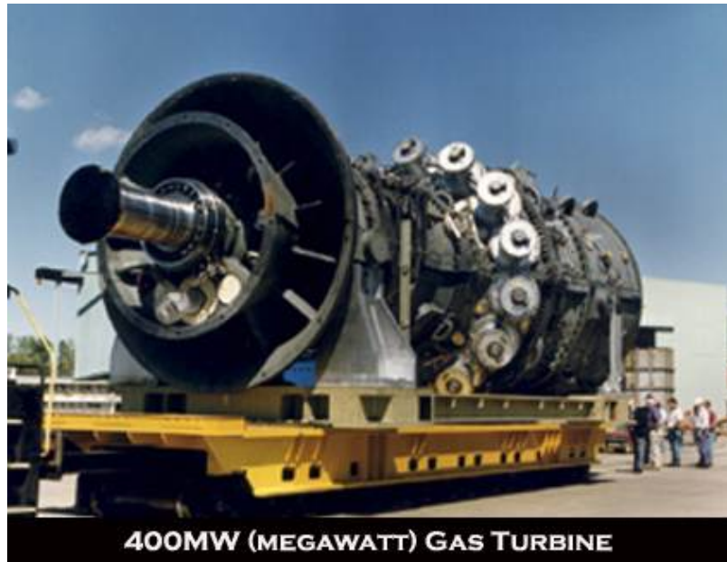
Figure 5-4: A modern gas turbine
