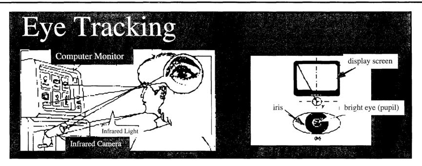
Low-power near-infrared source and camera provide eye look-point to  $\approx 0.3$  ° by comparison of corneal reflection (glint) and image of pupil center
