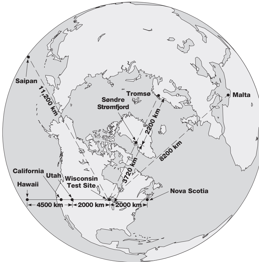
Figure 4-8 ELF propagation receiver sites for signals sent from the Wisconsin Test Facility in the Chequamegon National Forest near Clam Lake, Wisconsin.
