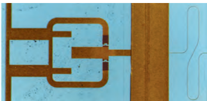
Figure 9-9 Monolithic gallium-arsenide 31 GHz receiver component showing a balanced mixer and metal semiconductor field-effect transistor amplifier on a 2.5 x 5 mm chip developed for an active-element phased-array transceiver.
