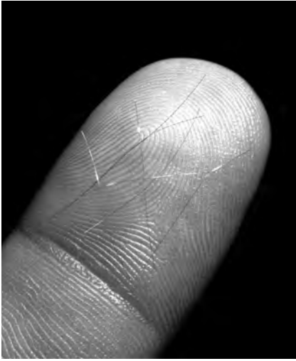
Figure 5-1 The Project West Ford orbiting dipoles were hairlike segments of copper wire.
