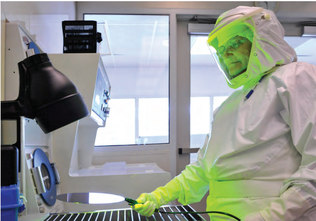
Figure 24-16 Microelectronics Laboratory staff with class-10 clean-room garment performs a bright-light inspection on a 200 mm diameter Si wafer prior to three-dimensional wafer bonding.
