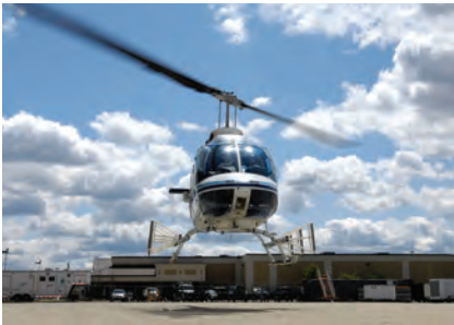
Figure 16-3 Bell Ranger helicopter with novel sensors attached to the landing skids.
