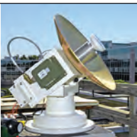
Antenna/pedestal system used on the Paul Revere to provide connectivity to Milstar
