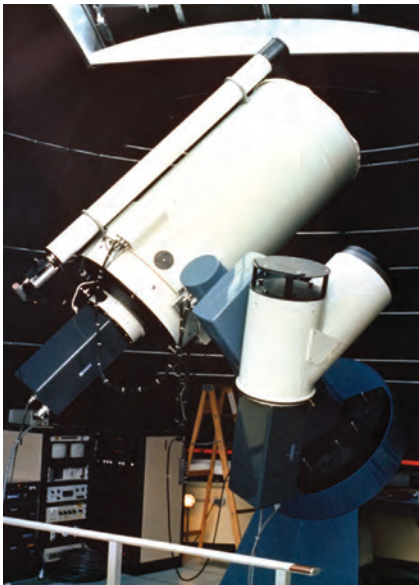
Figure 10-9 The 31-inch main telescope of the ETS with an intensified Ebsicon camera at Cassegrain focus. The 14-inch wide-field auxiliary telescope is on the declination axis, helping to counterbalance the main telescope.
