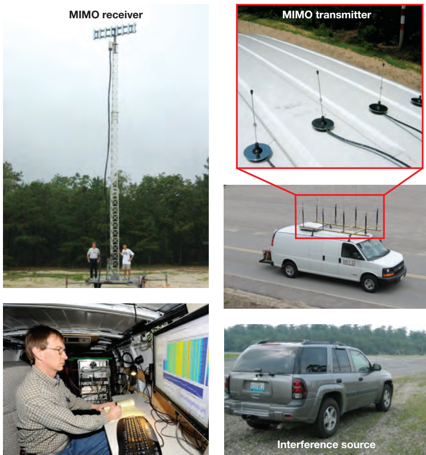
Figure 29-15 In this experiment conducted at Fort Dix, New Jersey, mobile transmit arrays and fixed receive arrays were used to test different waveforms and coding strategies.
