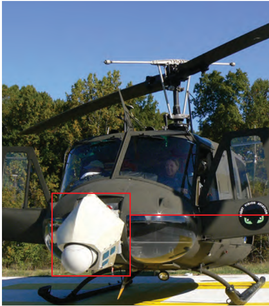
Figure 27-7 Phase 3 Jigsaw system. Above: The system is shown mounted on the helicopter. Right: A drawing of the system configuration and a cut-away view of the ladar optical head.
