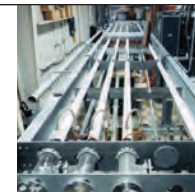
1000 W CW laser amplifier, Firepond
