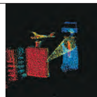
First collected imagery with a 1 \mu\text{m} sensitive APD array
