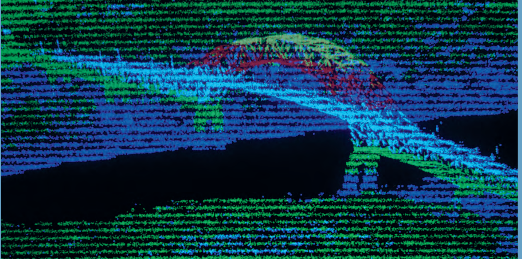
Figure 14-8 Laser radar image of the Bourne Bridge over the Cape Cod Canal in Massachusetts.
