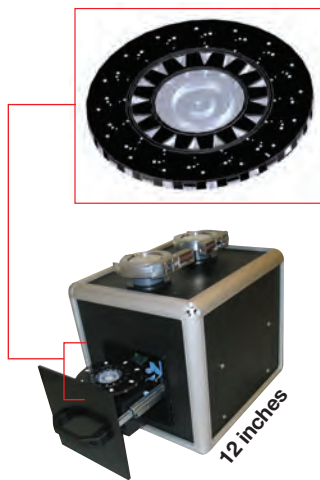
Figure 17-9 The portable PANTHER uses CANARY technology like the multiposition carousel shown in the top image, with the added advantages of automation, ruggedness, and reliability.
