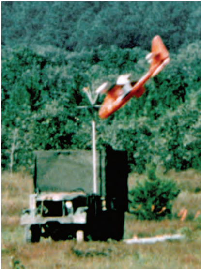
Figure 14-10 Direct impact of an antiradiation drone on the radiating antenna of a simulated tactical target.
