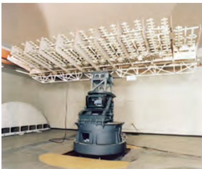
Figure 29-8 Radar antenna array for E-2C modernization program.
