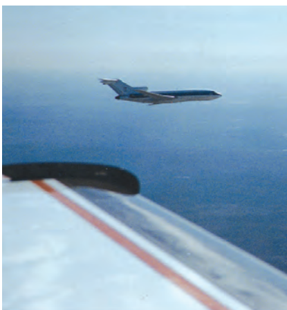
Figure 12-6 A Lincoln Laboratory test aircraft in a controlled encounter with an FAA Boeing 727 aircraft during TCAS testing.
