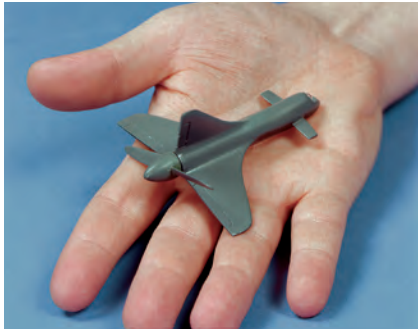
Figure 19-8 Model of a three-inch micro aerial vehicle.
