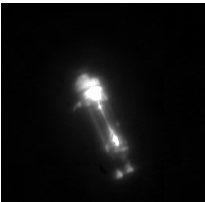
Figure 26-14 Images obtained at Kirtland Air Force Base, Albuquerque, New Mexico, with the Starfire Optical Range telescope. Top: The satellite Seasat at a range of ~600 miles; resolution is 10 inches. Bottom: Agena rocket body at a range of ~500 miles.
