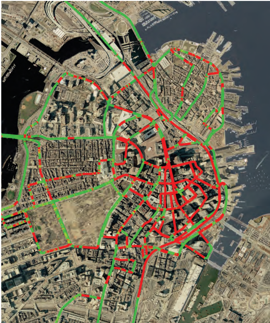
Figure 6-3 Result of a SATCOM link-blockage measurement campaign in downtown Boston. Green shows locations where the link is unobstructed and communication is possible; red shows locations where the link is blocked, making communication impossible.
