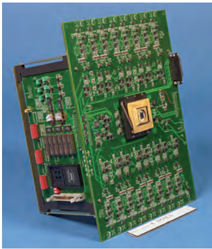
Figure 26-13 High-speed camera, using extensions of the SWAT technology, with a 128 × 128-pixel sixteen-output-port device mounted in a low-noise camera system.
