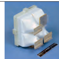
GEODSS fiber bundle with 4 × 4 CCD array aligned to upper right quadrant
