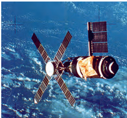
Figure 10-4 Above: Computer-generated simulation of a radar image of Skylab . Analysis by Lincoln Laboratory of actual radar images of Skylab (differing in detail and without the color enhancement) aided in understanding solar array deployment problems. Left: Photograph of Skylab taken after the remaining solar array had been extended and the crew compartment had been covered by a thermal blanket.
