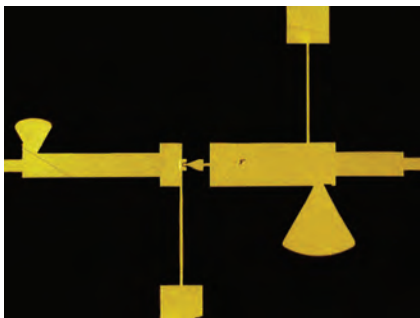
Figure 24-11 Monolithic Ka-band frequency doubler. A varactor diode is integrated with microstrip transmission lines, radial stub tuners, and bias lines. The length of the structure is ~3 mm.
