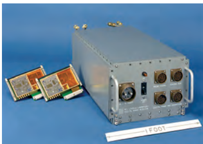
Figure 28-11 32-channel UHF-band digital receiver subsystems implemented using custom VLSI circuitry.
