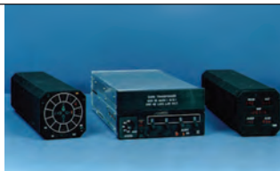
Prototype Mode S transponder and pilot display
