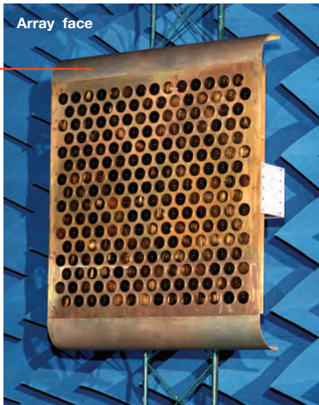
Figure 13-17 Top: DAR top-level architecture. Bottom: 224-element L-band DAR array in anechoic chamber.
