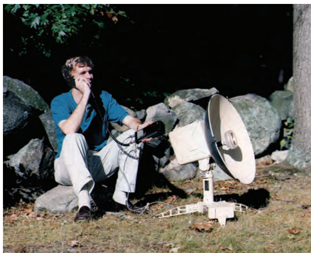
Figure 5-9 Clement Edgar is testing the Advanced SCAMP, a low-cost portable antijam satellite communications terminal. It is self-contained, incorporating an antenna, miniaturized transmitter, very-low-noise SHF receiver, and agile RF generator.
