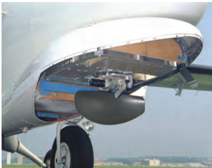
Figure 14-4 Paraboloidal dish antenna mounted in Amber UAV fuselage.
