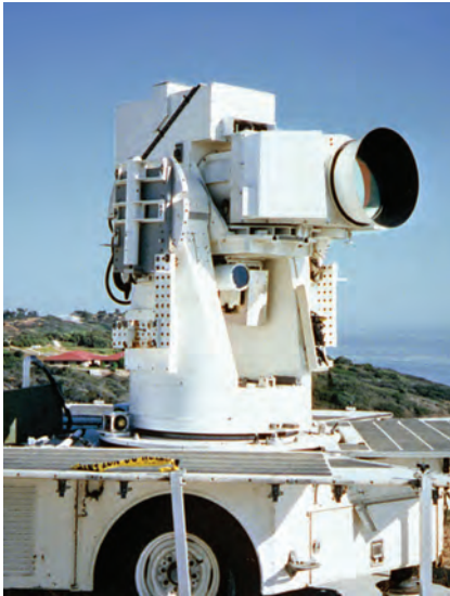
Figure 13-6 The IRMS sensor on a portable trailer mount at Point Loma, California, where it was used to characterize ocean surface glint effects.
