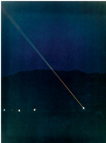
Figure 25-6 Sodium-beacon experiment at White Sands Missile Range, New Mexico. A 589 nm wavelength laser beam is sent skyward to generate a synthetic beacon in the sodium layer at an altitude of 90 km.
