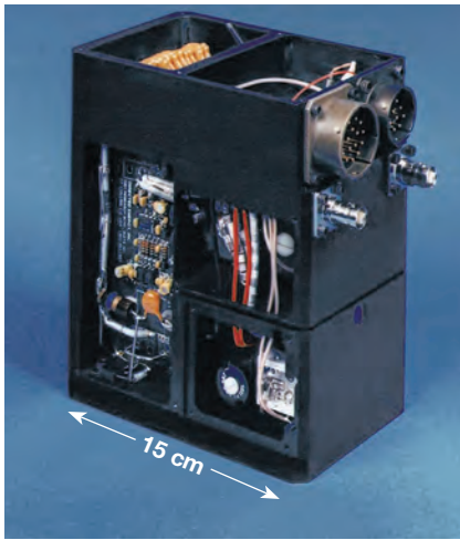
Figure 24-7 Photograph of an electro-optically Q-switched microchip laser system packaged for use in airborne light detection and ranging. The system shown contains the microchip laser, the pump diode, and all of the high-speed, high-voltage electronics required to Q-switch the laser. It generates 300 ps duration pulses with a pulse energy of 7 \mu J at a repetition rate of 5 kHz.
