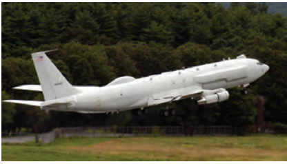
Figure 6-4 The Paul Revere aircraft is a heavily modified Boeing 707 that Lincoln Laboratory operates as a communications and sensor test bed.
