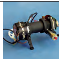
3-D ladar with scanning telescope, APD array, and transmit laser before integration into 12-inch gimbal for Jigsaw program
