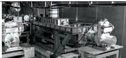
500 J single-pulse \text{CO}_2 lasers
