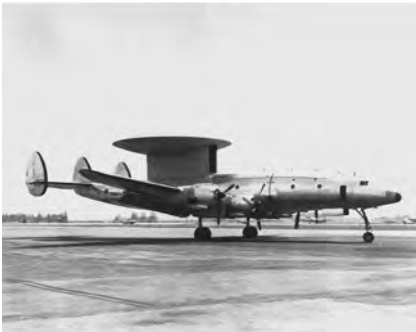
Figure 3-3 AN/APS-70 UHF AEW radar installed with its rotodome antenna in a Lockheed Super Constellation aircraft. This aircraft was the forerunner of the carrier-based Hawkeye and the land- based AWACS aircraft.
