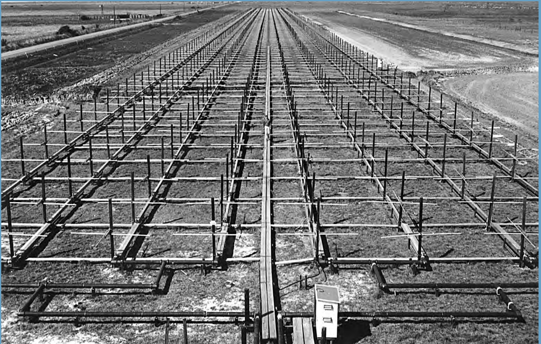
Figure 22-2 The 38 MHz antenna array for radar astronomy of the sun in El Campo, Texas. The scale of the array can be appreciated by noting the size of the individual in the center of the photograph.
