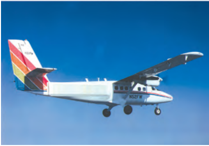
Figure 14-3 Flight test of the MASR on a Twin Otter aircraft. The displaced phase-center antenna is mounted on the starboard side.
