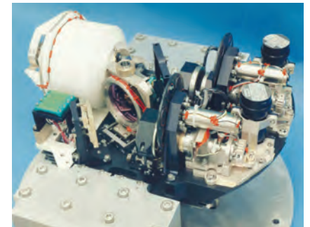
Figure 19-7 AIRI optical head including telescope (left) and detectors (right).
