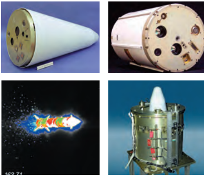
Figure 9-17 Clockwise from upper left: FASP, Midcourse FASP, FASP ejector module, FASP infrared imagery.
