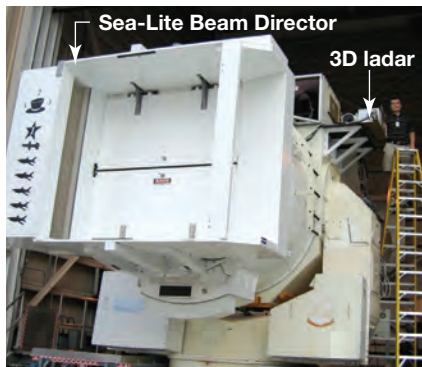
Figure 25-11 Three-dimensional ladar installed on the Sea-Lite Beam Director at the High Energy Laser Systems Test Facility at the White Sands Missile Range in New Mexico.
