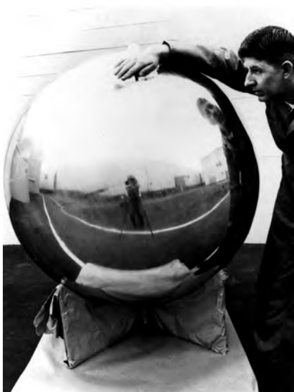
Figure 10-3 The Lincoln Calibration Sphere prior to launch. Although the sphere was designed to be used for radar calibration, the highly polished surface also allowed its use by optical sensors.
