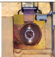
Laser diode array for first wavelength beam combining
