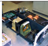
3-D ladar operating at 1.5 \mu\text{m} wavelength
