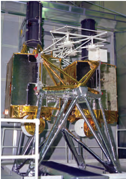
Figure 5-5 LES-8 (left) and LES-9 (right) assembled at Cape Canaveral Air Force Station, Florida. The satellite assembly was integrated with the Titan-IIIC booster.
