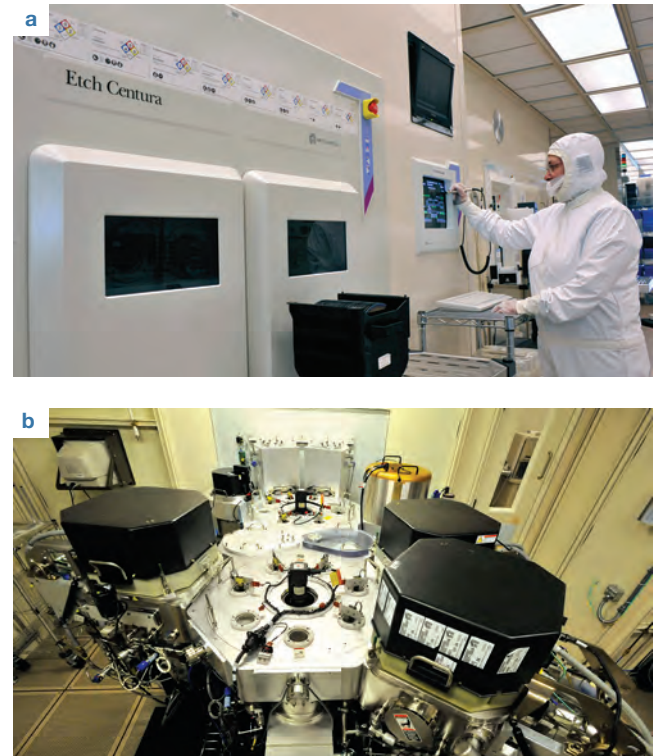
Figure 24-17 (a) Cluster plasma-etch system viewed from clean room. (b) Physical vapor deposition system viewed from clean-room return air chase.
