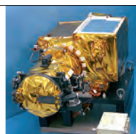
CCD focal plane for SBV telescope
