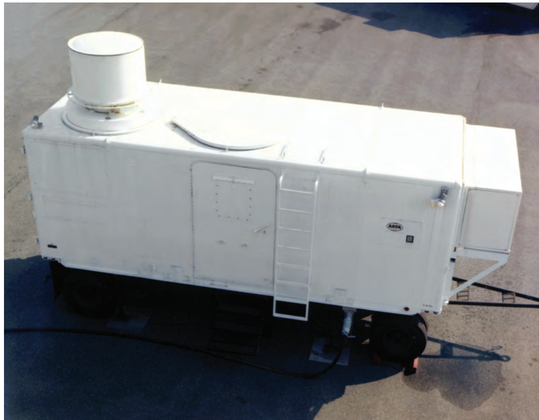
Figure 14-6 The AGSR, a cylindrical phased-array antenna integrated with a PMP.
