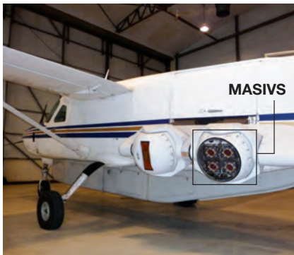
Figure 15-4 MASIVS mounted on the Cessna aircraft.
