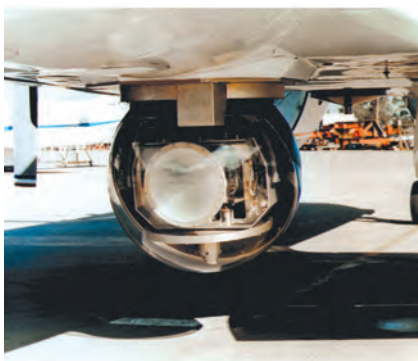
Figure 14-5 Fully polarimetric, high-resolution SAR mounted below the fuselage of a Grumman Gulfstream G-1 aircraft.
