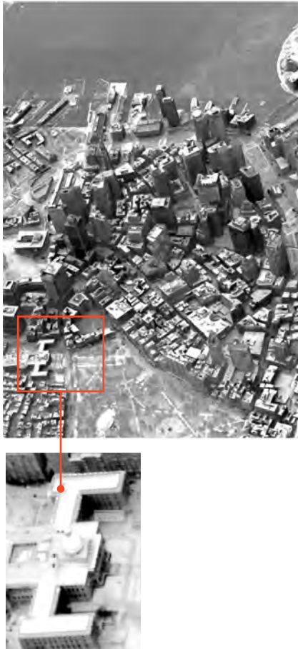
Figure 15-5 Aerial, winter night, infrared image of downtown Boston collected by a camera using the digital focal-plane array. The inset image of the Massachusetts State House partially illustrates the detail present in the image. Infrared image resolution is less than 1 meter, and the image quality is better than a high-definition television image.
