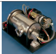
Infrared countermeasures optically pumped 4 \mu\text{m} laser
