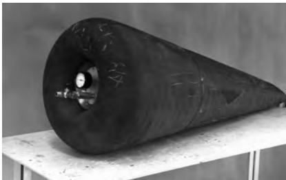
Figure 9-7 Inflatable ballistic missile decoy developed by Lincoln Laboratory.
