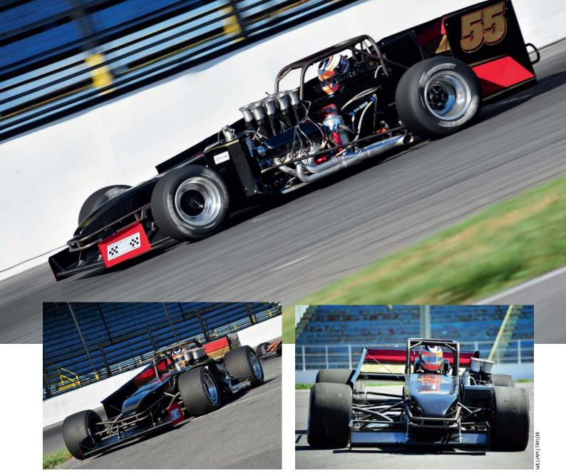
The cars feature no transmission or gearbox, and the engines drive the rear wheels directly. If a driver spins, that spells the end of their race
