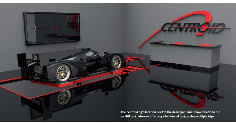
he rise of simulation technology in motor racing, both multibody and driver-in-the-loop, has placed ever-increasing importance on understanding a car's real moment of inertia and centre of gravity. The first test rig to be revealed that is specifically-built for this task was revealed in 2012 at Cranfield University in England.
