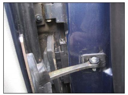
Pull the door connector holder toward the outside of the car, and separate the two halves by levering up the end slide.
