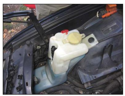
**Step 2. – Install tank**Slide the intensive cleaner tank onto the regular washer fluid tank.
