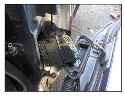
Pull the inside connector out through the bodywork hole, mate up the two connectors, and then look and feel in the back of each one to make sure the small connectors are fully seated with each other. The key is to test operation before putting everything back together.
