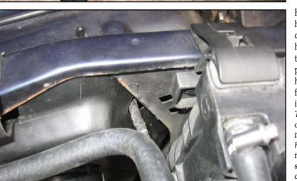
If you go high, run the harness forward in the area at the top of this picture, where the grey connector is (that's the side marker connector, not in its normal place). There should be another hole to put another harness-holding clip in.
