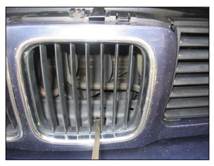
With the ends of the center grill loose, depress four catches near the "kidneys" in the middle of the grill. The two at the top need to be pulled up slightly; the two at the bottom pushed down (through the grill). Then you can pull off the whole center grill / trim.
