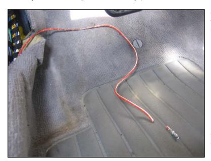
Crimp the two same-color wires together on a new larger male connector pin, 61 13 1 376 195.
