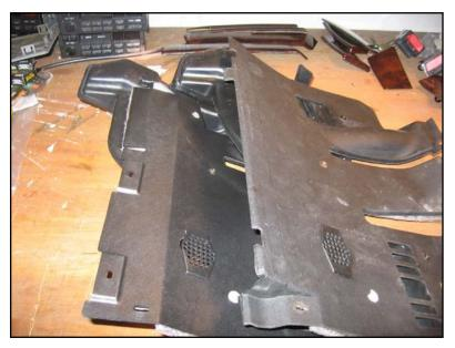
Replacement trim panels are needed for lower dash areas left and right of the steering wheel, and also a new foot pedal cover is needed. Although the U.S. and European versions of the latter are similar, they are not interchangeable since the profiles of the trim panels are different, and they meet the pedal cover panel at somewhat different angles and locations.
