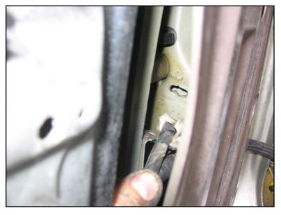
Once the box pathway is clear, disconnect the harness from the various holders on the inside of the door; if you can figure out how to get the wire out of the holders, fine (one on top of the clip you can see by peering into the door; two others flip open; a couple you can push out of the sheet metal from the outside of the door), otherwise break off the holders by pulling/prying them or the harness itself.
