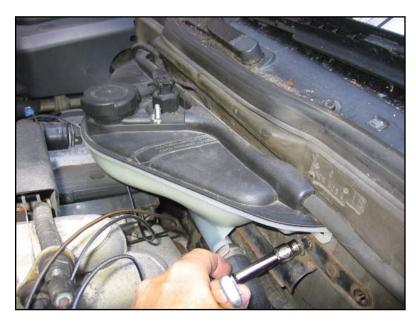
Remove the nuts holding on the coolant expansion tank, then the nuts holding on the metal wire channel underneath it. Zip tie the wires to the channel, as the existing harnesses are.
