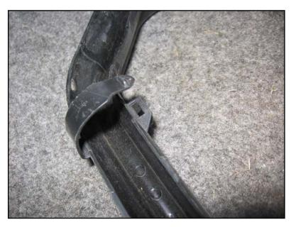
Tabs on wire channel pop out; watch out, one of mine was broken off.
