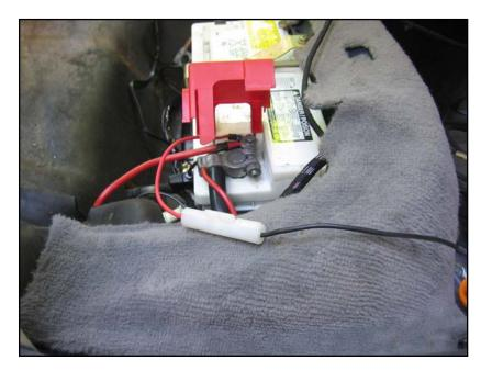
Run a 1 mm<sup>2</sup> or larger wire from the battery positive post through an in-line fuse holder to the relay connector and crimp on a contact. Strangely, my car came with such a wire and fuse holder already attached to the positive cable, probably aftermarket.
