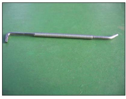
Middle of tool is a spring that allows tensioning of the adjusting cam without turning it, by applying just the right amount of pressure.
