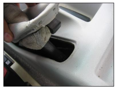
Push rear of handbrake gaiter assembly forward gently, and up, to release this catch.
