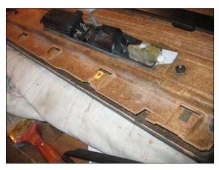
The slots for the speed nuts can be nicely cut with a circular saw. The slots should ideally be cut where the bottom of the speed nuts will lie, which depends on where the screw for the speed nuts goes, which, in turn, depends on where the shade itself lies. I lined up the shade evenly with the top of the adjacent fiberboard horizontal section. Align the saw carefully, and don't slip.
