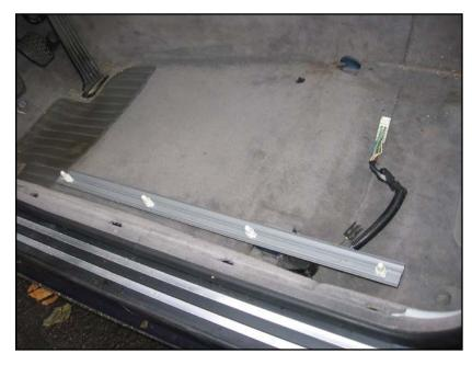
Left front door sill trim – lever it up gently, right next to the clips, with a large screwdriver.
