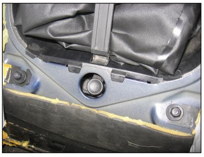
Rest the bottom tabs over the edge of the sheet metal and snap the top clips into place. The top clips did not go on easily in my case, but checking the alignment from the passenger compartment side and pushing and pulling firmly did it without breaking anything.
