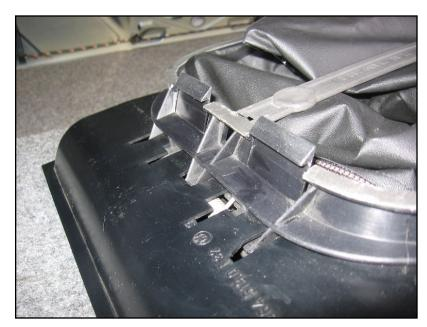
At the top, make sure the tabs on the frame go into the right slots of the ski sack assembly – if you're forcing it, try the other slots.
