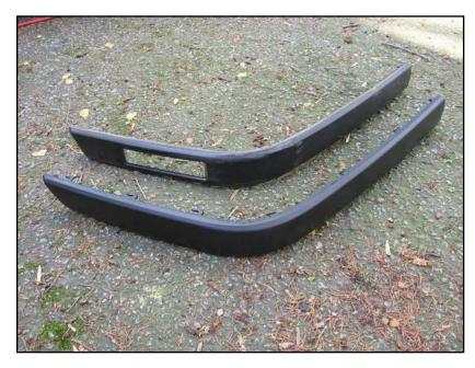
A U.S.-spec bumper trim (for the car's front right) is at the rear; European-spec is to the fore. Front of the trims are to the right.
