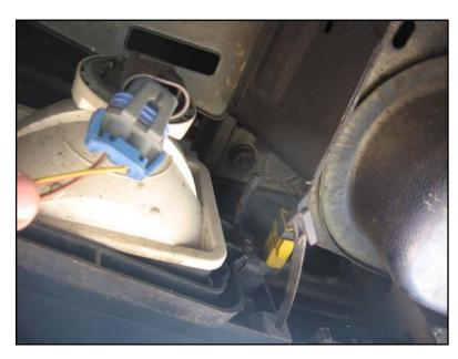
Separate the fog-light connector, and twist out the outside-temperature sender from its socket.
