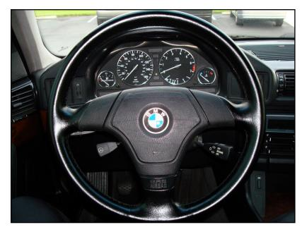
D. Here is the 1995 3-spoke design, also found on some M3s. It too came in a rare wood-rim version. It fits on the '95 models; earlier models need modification of wiring. Note that some later wheels (on various '99+ models) look just like this but use an incompatible airbag, with a dual-stage system. The connector on the back of the later units is a yellow 4-pin type, rather than the earlier orange 2-pin type.
