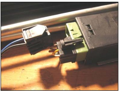
Disconnect the motor wire connector from the control unit.
