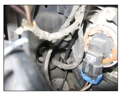
There are a couple of grommets to go through, for a stock look. One is buried in front of the radiator. Take off the trim panel behind the headlights (two clips turn 90°); it's much easier to take out the air filter housing first. It is very difficult to feed the new wire through the grommet in place, so pull out the grommet and slide it up its existing wire so you can reach it to push the new wire through.
