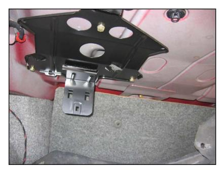
Plate held on by three brass-colored bolts in pre-threaded holes. Wire-holding clips go in the tab sticking down at the back.
