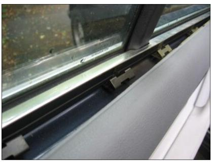
At the top of the door panel, a vertical flap of the underlying fiberboard fits into clips underneath the chrome strip. To remove the door panel, first ease the top of the panel and these flaps out of the clips, pulling slightly in towards the center of the car and then upwards.
