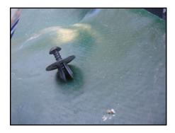
The mat attaches with numerous clips. Unscrew the screw to allow the rivet to be pulled out.
