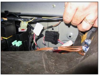
Note that a small second, adapter wire loom may be needed if the car does not have the appropriate vehicle wiring already installed. If the wiring is already installed, part of it will be underneath the rear seat base, on the front wall of the seatwell, to the right front of the rear fuse box. Look for a black sixpin connector, **X269**, probably behind a white four-pin connector (the latter is for rear seat heating/headrests).
