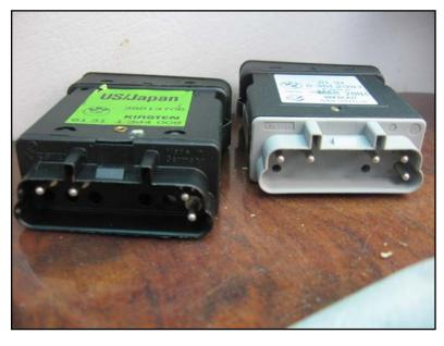
Front-only fog-light switch on the left, frontand-rear switch on the right with the extra pin (number 4).
