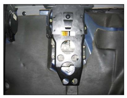
Be very careful, don't overtighten the sheet metal screws when installing the brackets to the bulkhead, the bolt holes strip very easily! If a bolt hole does strip, it should be possible to rescue the situation by using a speed nut – as is already done for the lowest of the three holes – after cutting an insertion hole for it.
