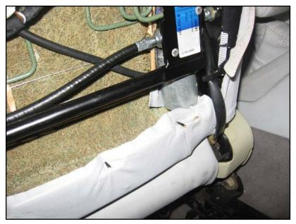
To get the seatback off, use adjustable groove joint (also known as "water pump") pliers to pull down the spring-loaded levers. The right-side one is shown in the picture (grip the lever and the frame below it, squeeze them together). There is one lever on each side – lift one side a little then release the other lever and lift that side, but don't twist things out of shape. Someone suggested it's easier if you disconnect the spring first, but it's usually not necessary.
