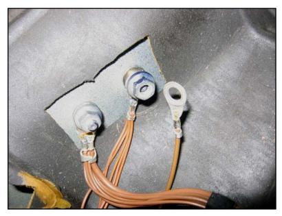
and connect the ground wire to a suitable ground terminal stud;
