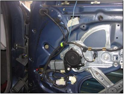
New tape-wrapped mirror harness coming down along the existing passenger-side door harness, looping around underneath the window motor to take up slack, and heading forward out the front of the door.
