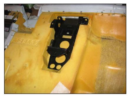
This shows how the brackets lie in the seatback foam once they are attached to the bulkhead and the seatback is put back in place.
