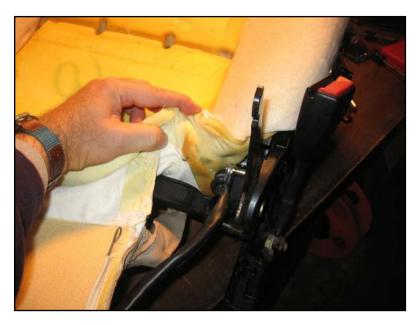
There may be a couple of hog rings to attach at the rear, holding the cover directly to the foam.
