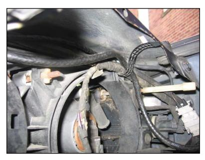
Secure the hose under the sheetmetal at the top front of the engine bay, using the existing wire and hose straps.
