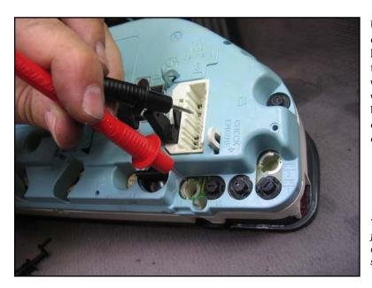
Use an ohmmeter to check for continuity with the right side (when looking at the cluster from the back) of the empty bulb socket for the rear fog warning light. Mine was pin **X502/15**, which was the second pin from the bottom on the left side of the connector socket, looking at the back of the cluster.
