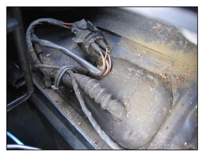
In theory one could crimp on the extra wire at a new pin on the wiper connector, **X333/4**, out in the plenum, but that would be tricky since the pins at the wiper connector are waterproofed.
