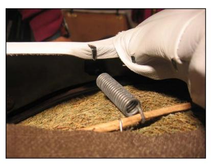
Remove the leather covers from the seat base and from the seatback by stretching the leather off the metal prongs on the seat metal. (Careful, some of the prongs are sharp.) A few prongs may be bent down, and may need to be bent up to ease the leather removal.
