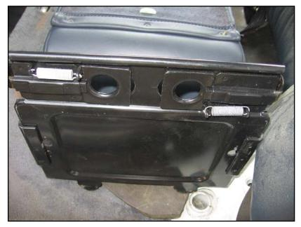
Cars up to about 12/90 build date used the early-type of armrest. This was held in by a quick-release bracket similar to that used for the E34 ski-sack armrest (see that chapter), but this bracket is much shorter, so the brackets aren't exchangeable without modification of the seatback.
