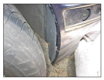
Pull the trim inside the wheel well clear of the bumper ends on the sides.
