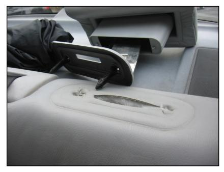
Put the seatback in place and carefully locate where to make cuts in the leather for the headrest's flat shaft and a trim plastic screw on either side. Hold the lower trim piece where it will be inserted and mark the leather. You can also feel for the metal bracket slot and holes at the top of the seat through the leather. Do this all very carefully because if you cut in the wrong place, it will show. Cut small holes/slits at first, and keep checking them as you expand them.
