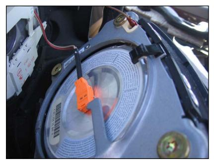
Disconnect the airbag and horn connectors.
