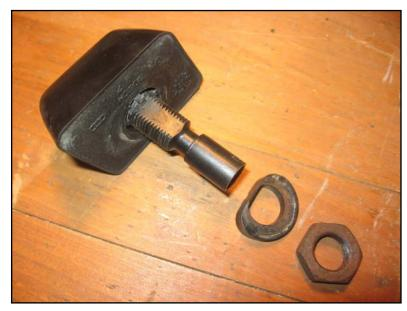
Install headlight nozzles in the top holes – left and right nozzles are different.<sup>23</sup> Put the lug in the notch you cut earlier. Use the metal, not plastic, nuts.
