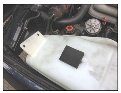
Attach the foam pad on the back side of the tank.
