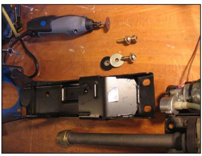
Since I did not have power at the yard and was having difficulty hacksawing, I used another method: I simply undid the pedal bracket, to which the steering column bracket is attached, and removed them together (see earlier picture for the five nuts and bolts); also remove the clip holding on the brake pushrod clevis pin, and release the accelerator. Back home, it took but a few moments to cut a slot with a Dremel<sup>®</sup> tool, and loosen the bolt, turning very hard with a large screwdriver.
