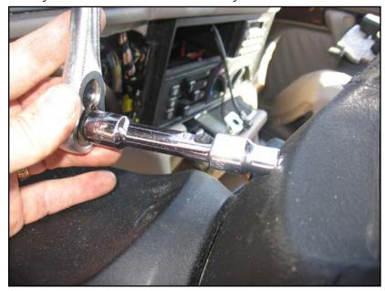
Take off the airbag – two T30 captive bolts at the back of the wheel.
