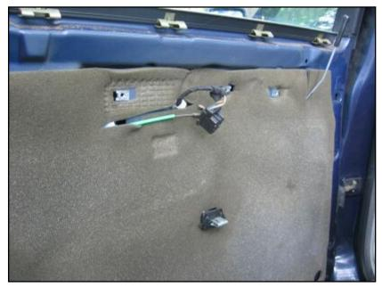
Gently lever the window switch out, then disconnect the connector.
