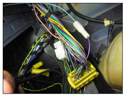
Wire 1. Splice a wire from the Raintronic control module terminal 15 to the **vi/sw** .5 mm² wire already going to **X14/9**, or merge and crimp the wires at a new pin connector in the 9 slot. I did the former. (On a '92 the existing wire brings power from fuse 24 to the general module, **X255/10**, under the rear seat.)
