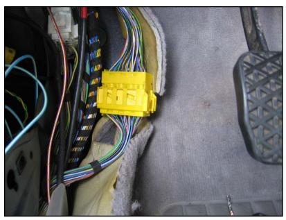
The connector that the wire normally runs to is not in the speaker cavity in the sheetmetal or high up, but behind the floor carpeting in the front corner of the footwell. It is connector **X14** (yellow, 30-pin in a '92).
