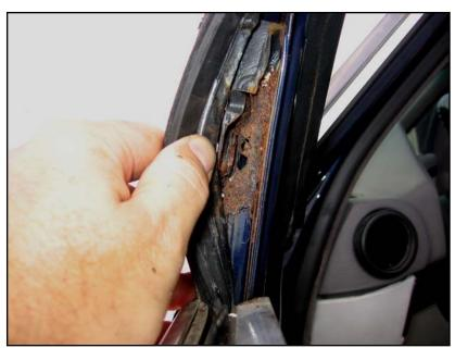
Apparently the three pieces of foam packing in the door and mirror don't do much to keep out water – and may even form a water trap, given the extent of rust I saw.
