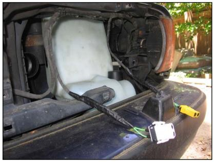
Finally, wrap the wires in fabric tape.
