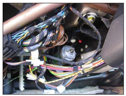
Take off the pair of bolts toward the front of the steering column bracket.
