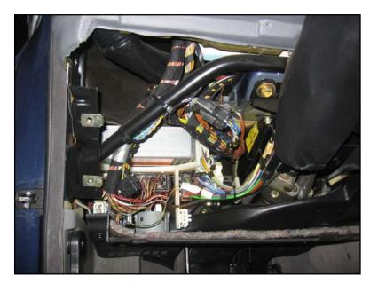
Unscrew the screws on the center console and remove the right trim panel. Note which screws go where on the center console.
