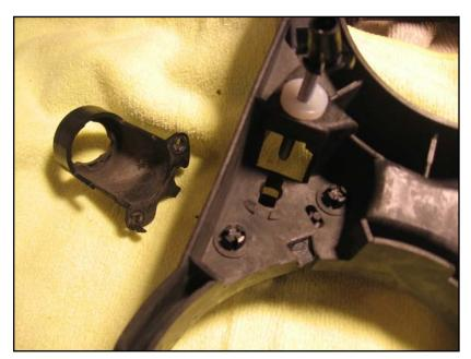
A strong word of warning on old adaptors: the prongs that go into the headlight plate are *extremely* fragile, and once the prongs break, there's no way to mount them and, hence, the motors. Do not take out or insert the adaptors and motors unless you really have to or you have new adaptors available.
