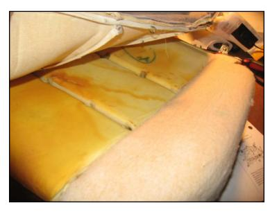
The leather seat covers have thin metal rods, in cloth sleeves that are sewn to the leather at the seams along the side and transversely.
