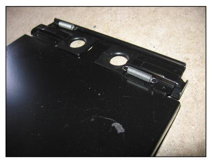
Step 5. Attach quick-release bracket latches to seatback
