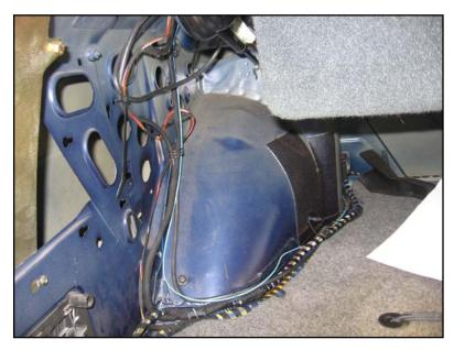
Lay the wire to the light assemblies, inserting it in the existing harness clips or using zip-ties, leaving slack by the hinge as needed.
