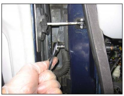
Detach the door connector from the door jamb by unscrewing the trim holding the rubber tube and grommet. You will probably be taking off the door (in order to reinstall the connectors easily – see the discussion further on). If so you might want to do it first, it's much easier to unscrew the connector trim bolts with the door off.
