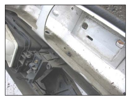
Remove the plastic rivet pins along the front and bottom sides of the bumper carrier, from the inside. Careful not to mash a pin if it's tight.
