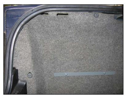
Remove the left-side trunk carpet after turning the two clips.
