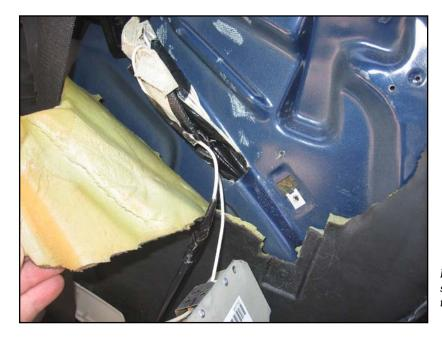
Left-side mounting area showing the speed nut (silver rectangle) in place for the lower bracket screw.
