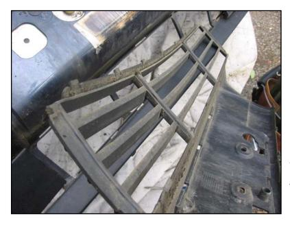
Lugs at bottom of center trim and grill. There are also three at the top of the grill portion (right side in this picture) that are hard to see here.
