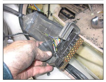
Cut open the rubber casing at the door connectors to liberate the wires. Keep the woven fabric sleeve on the needed wires by cutting the unneeded ones and sliding them out of it.
