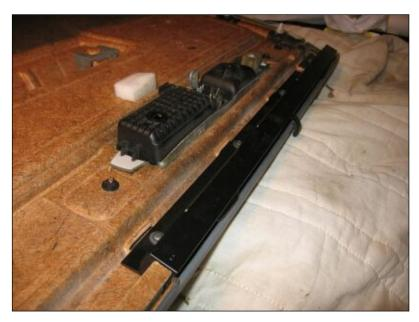
Step 7. – Attach roller to door panel
