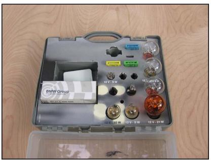
The fuses and the top two bulbs in the picture were not in the original kit, but sockets were in place under the cover sheet to hold them. Other spare locations to hold bulbs are also visible.
