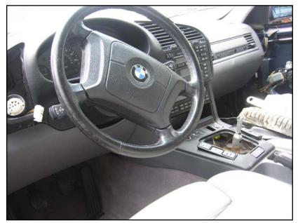
C. This is the 1995 (5/94+) new standard design with a nice colored roundel (shown in an E36 here). Notice that the accent ridges line up along the center of the spokes, as opposed to the earlier design where the ridge along the top of the airbag lined up with the bottom of the upper spokes. The wheel also came in some beautiful wood-rim versions.
