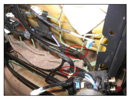
Zip-ties for lumbar (top red circle) wires and for harness coming up from the seat base (bottom circle). Find similar locations if using a different seatback frame. Note the white tape around the harness by the lower zip-tie. The factory usually uses these white tape markings on the black harnesses to show where a zip-tie or other holder goes.
