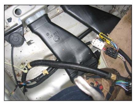
Supplementary-harness to vehicle-harness connector was actually located underneath the air ducts, as shown here (just visible behind the yellow connector), not on top as in the earlier picture. Note the connectors that go up to the seat, at right in the picture (top three plug into control module; lower one in bottom right corner of picture plugs into another harness on the seat). Also note the white zip-tie wire holder on a stud at left, with a useful, all-too-rare release tab!
