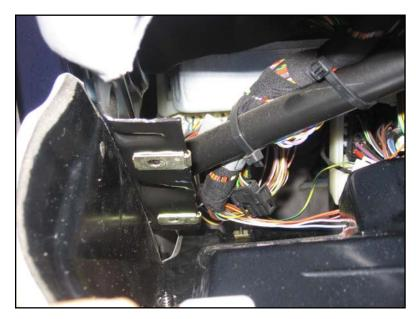
View looking down past a slightly-pulled out dash trim. The back of the driver's glove box is the black shape at the bottom right of the picture. Knee-protector flange has the large speed nuts on it. Dash brace is the large round bar with the zip-ties.
