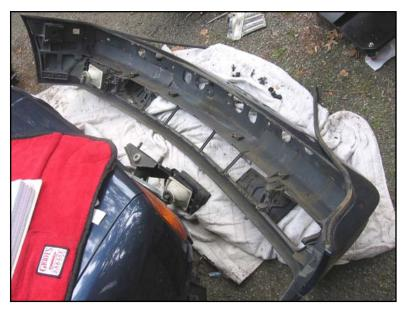
Remove the metal bumper carrier from the plastic bumper cover.
