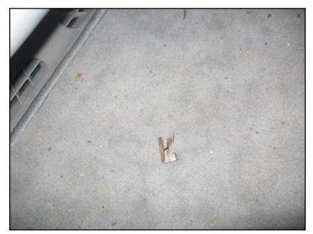
Remove the two clips holding the green zigzag rod to the wrapped wire lattice (see picture). The clips were very strong and needed quite a bit of force to be pried off. The EBA doesn't say it anywhere, but in a factory-installed lumbar support, the clips attach the rod to the lattice too, just as for the fixed wire support. If desired they could be re-crimped on for this lumbar installation.
