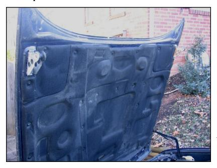
Remove the insulation on the underside of the hood by unscrewing the plastic screw in the clips, far enough to be able to pull out the clip. There's lots of them, and the screws can be surprisingly sticky for plastic, so be careful not to strip the head. Some replacements are inferior, having even smaller screw slots. Some early cars had a better clip that is released by levering out the center pin.
