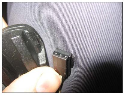
Wire connector on a mirror. Note that this shape, including the tab, does not mate with the '92 connector on the car. For my application, I needed to cut the tab on the right side off.
