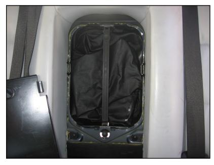
Insert the ski sack into the passthrough opening.
