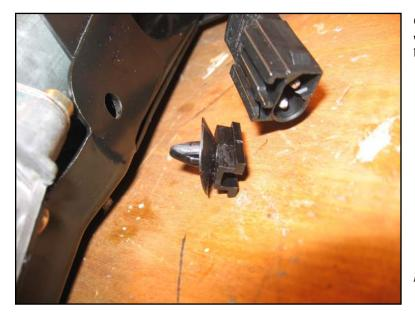
Once the bolts are in, clip on the motor wires using a clip on the side of the bracket.
