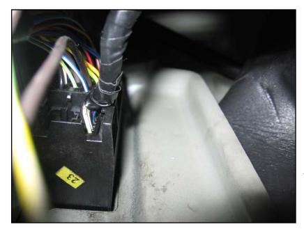
Success: this shot from inside the footwell cavity shows the inner small connector (with wires wrapped in electrical tape), large connector (at top), and outer shell in position and all mated to their outer counterparts.
