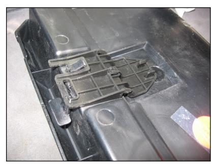
A single plastic clip is needed to hold the kit in place on the underseat bracket.
