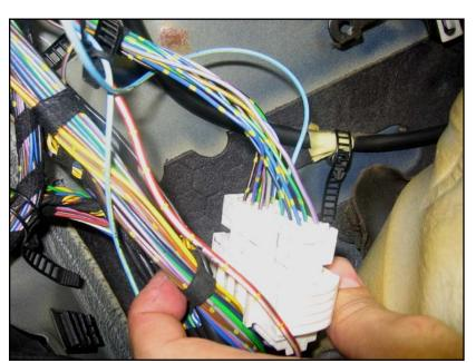
Once the inner portion is moved slightly, crimp on a contact and insert the wire into the pin 5 hole.
