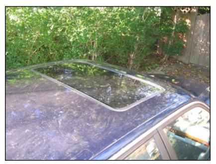
Slide in the sunshade through the sunroof opening, toward the front, then slide it back into the headliner out of the way.
