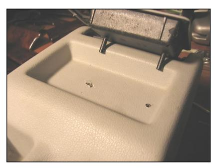
Drill holes for the studs of the add-on switch plate, which serves as the new storage tray.
