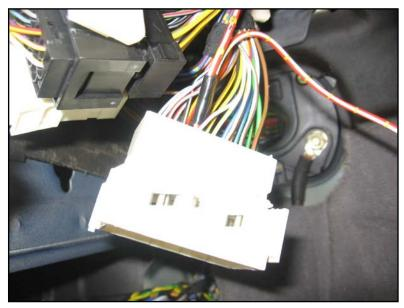
Insert the new pin into the correct pin hole until it clicks into place.
