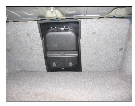
Note the two round magnets at the bottom of the ski sack cover, which stick to the ceiling of the trunk when the cover is open.
