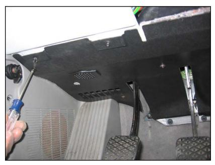
Screw the pedal cover to the bracket at lower left, and to the brackets at the front of the footwell.
