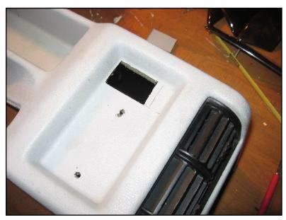
The switch cut-out viewed from the top. The pre-cut hole in the underlying plastic doesn't actually go as far towards the rear as the cut dimensions in the EBA show. You don't want, or need, to cut as far as the EBA says, so just cut to the edge of the plastic hole. The partial cut line that is not too visible in the picture was cut from the top before I realized the plastic hole was pre-cut underneath.
