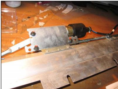
For reinstallation purposes, mark the edges of the three phillips screws holding the motor to the shade frame; unscrew the screws; and remove the motor. (You actually can leave the motor in place on the shade frame if you like, but it makes things marginally more accessible to take it off.)
