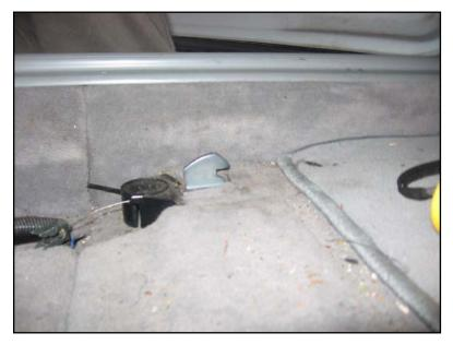
Refer to the shape of the hooks on the car floorpan that hold the front of the seat in place, shown in the picture, so you can get an idea of how the seat needs to be moved to get it off.
