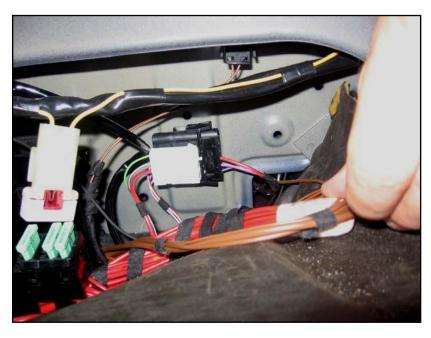
Vehicle wiring for the headrests terminates at the white 4-pin connector in the middle of the picture.
