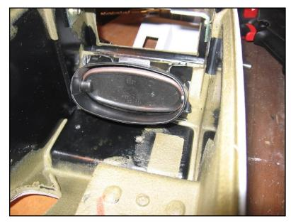
This is the underneath of the rear console. The tan rectangular area within the black plastic (to the lower right of the oval air vent in the picture) is where the cut-out hole for the sunshade switch goes, so it's easiest to cut through from this side. As with many items, BMW designed the console prepared for accessory installation.
