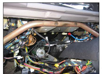
If you're removing the pedal bracket too, pull down the steering column slightly and access two remaining bolts.
