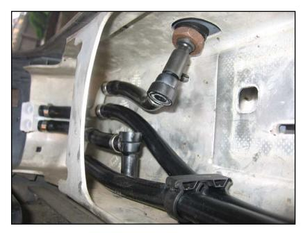
Clip the white distribution block into its hole on the left side (for the 535i – many other variants use the right side; reverse things as necessary) of the bumper carrier. Coat the valves with glycerine and insert them into the nozzles. Insert hoses into the hose holders, and into the c-shaped plastic brace if not already done.
