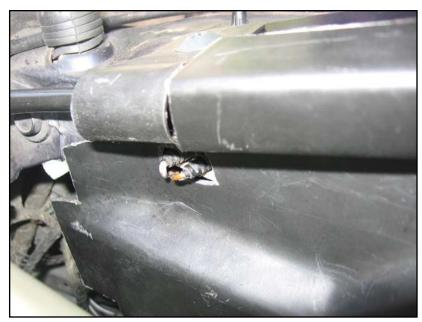
Strangely, since the factory is so good at integrating such things, on the left side, the trim behind the headlights didn't seem to want to accommodate the city-light connector. Cut out a small hole if needed. The right side was close, but seemed okay.
