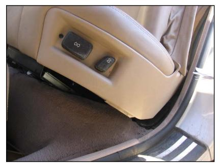
The switches for the E32 rear reclining seats included a headrest raise/lower function that would adjust the headrest height and override the automatic control. They were on the front corners of the seat base. The E34 switch is in a similar location, but of course only includes the manual headrest raise/lower function.
