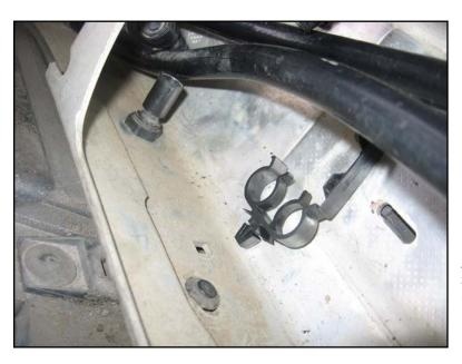
Fog-light nozzle installed. It is secured to the metal bumper carrier, not the plastic bumper cover. Note the hose holder that will be clipped into the nearby square hole, in the next step.
