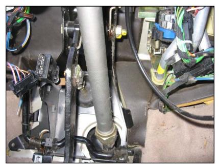
If the donor is an automatic, cut the shift interlock cable that is screwed in near the ignition lock.
