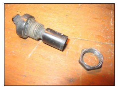
Install the fog-light nozzles in the bottom holes. Lug into notch again. Use the plastic, not metal, nuts.
