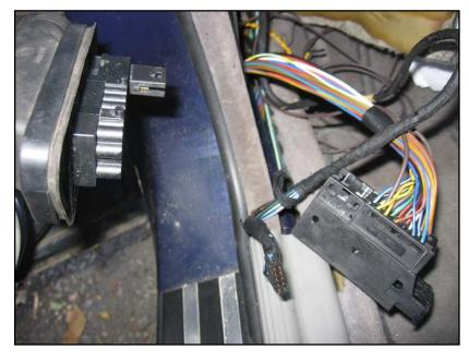
You might get lucky after several tries; if you fail, try this: take the male-male pin connector piece off the inner harness small connector, and put it on the outer small connector.
