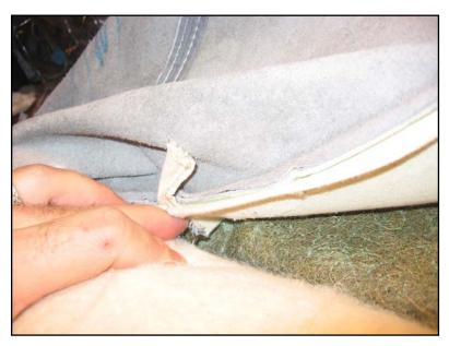
At the ends of the lateral rods there are short strips of cloth that are glued to the foam and need to be released.
