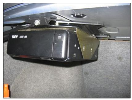
The Pioneer CDX-M90 changer attached to the left ceiling of the trunk. Note the three mounting plates: the greenish one on the changer, a black one in the middle secured in part by the prominent bolt in the picture, and a top black one along the trunk ceiling.
