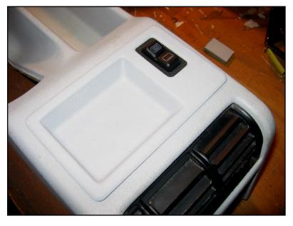
Install the trim plate using the spring clip washers. Reinstall the console, bringing the switch wire up through the switch hole. Connect the wiring to the switch, and then install the switch.
