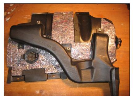
If needed, transfer the gong cover, air duct, and duct grill from the old panel.
