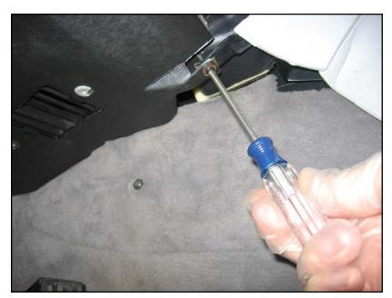
Screw the pedal cover to the two trim panels – three screws along the top of the cover.
