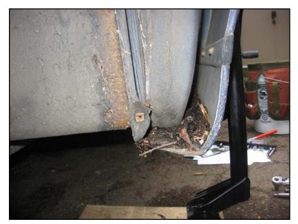
Once you take off the liner, you may see a bunch of decayed plant matter etc. in the nice fender rust trap. While you're here, clean it out – and do the right side of the car when you're done with this whole installation!
