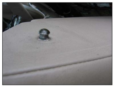
Shown here is one of the side pins that pop out of the bracket when taking out the late-type armrest. The armrest pin simply pulls out past some springs in the bracket.
