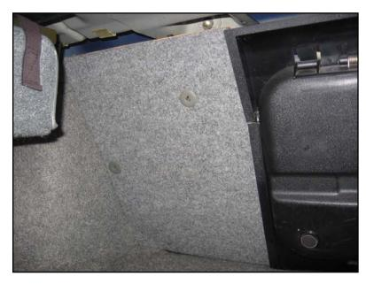
Remove the insulation panel on the trunk side of the bulkhead with a screwdriver in the plastic nuts with the odd-shaped holes (see chapter on ski sack).
