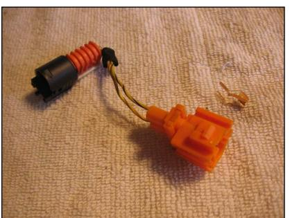
The airbag connectors were different between my '92 and the '95. Proceed at your own risk since this is an important safety item, but I took the old wheel-side connector and attached it on the end of the new vehicle-side connector wires. I slipped the wire contacts out of the existing connector using the special contact-removal tool, crimped new contacts on the end of the donor connector wires, and inserted the newly-crimped contacts into the existing connector.
