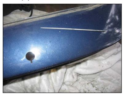
Cut the notches for the lug on the headlight nozzles – 5mm out from the circular hole, 3mm wide. The first one I did painfully slowly with the mini-file seen in the picture. The second one I did in 8 seconds with a reciprocating saw – cut very carefully if you do the second method!
