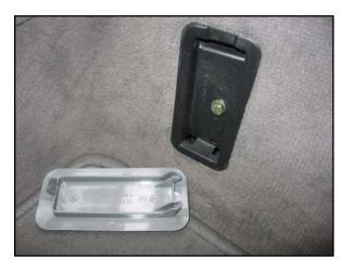
Remove the battery negative-disconnect covers (did you know that's what that was for – you don't need to take off the rear seat base to disconnect the battery!).
