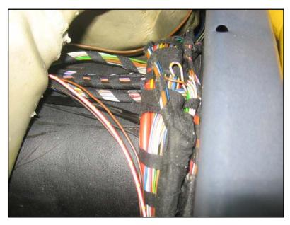
Slide the section of the wiring harness leading to the seat-heating switches underneath the carpet, alongside the other wires, forward to the center console.
