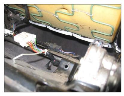
This is where the main white seat-tovehicle connector, **X275**, is zip tied underneath the seat, toward the rear (nonmemory only).
