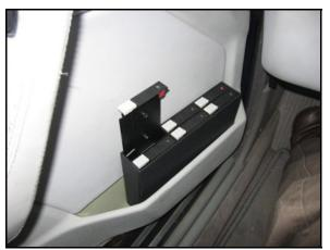
Cassette storage box. A red dot (barely visible on furthest tray in the picture) appears when a cassette is in the tray. Tray releases by pushing on the light gray button.
