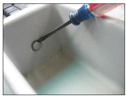
Rear console screw cap in storage bin. Could also use a pick to pull it off.
