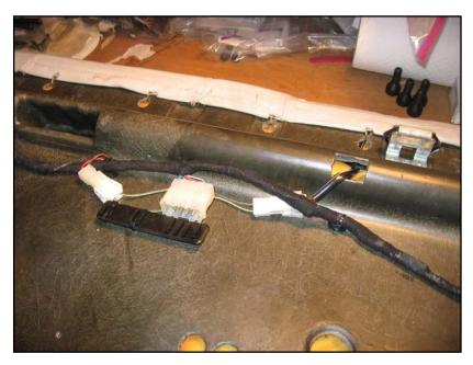
There was an unused square hole on the left side of the seat base, so I ran the wire lead from the cover, between the hard shell of the seat base and the seat foam, and out the hole. Possibly that might help the lead not getting pinched where the seat rests on the footwell wall. There wasn't a similar hole on the right underside, so if desired one would need to be cut.
