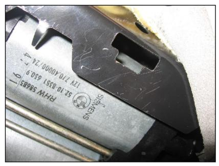
This is looking up from underneath the front of the seat, which is toward the top of the photo. The tab with fixed nut on the extinguisher bracket fits up into the rectangular hole shown, and the bracket bolt goes through the circular hole just visible under the leather at the top right in the photo. Note the hook that holds on the leather, to the top left in the photo.
