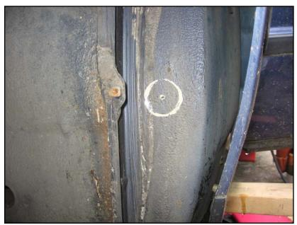
Now do a test punchmark from the wheel well side, in the center of where the harness hole should be cut. Then from the footwell side pull back the foam covering at the front of the cavity and feel for the punchmark. Check that the forthcoming hole will be in a good place, i.e., doesn't hit the sides of the cavity and is at a good height, ideally near where the zig-zag cut in the cavity foam is.
