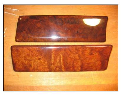
Oddly, the wood trims on the European and non-airbag panels are very slightly wider than the U.S. ones and have very slightly different shapes (mine were marked "ECE", for Economic Community of Europe, on the back).
