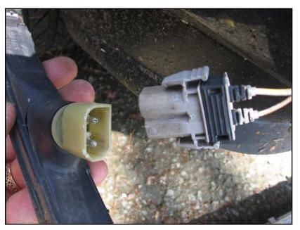
To plug into the vehicle side of that connector, I ran the new wire to a factory connector half that matched and replaced the side-marker-light side of that connector.
