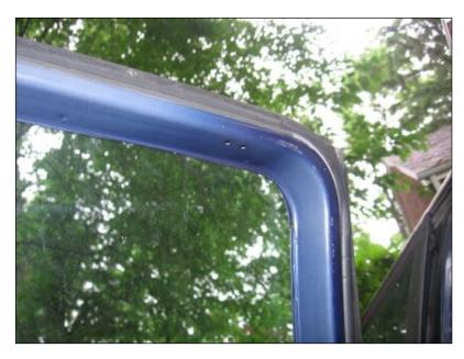
Predrilled holes for main shade fronthook screw and alignment lug (i.e., not for two screws).
