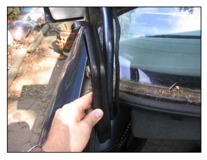
Carefully unclip the wire channel that goes along the curved trunk-lid arm.
