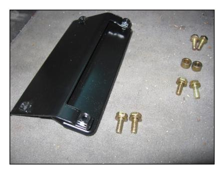
The installation kit. The bracket is facedown, showing the rear side with the tabs that go in the seat. The two spacers are not needed for standard seat installation. The kit comes with two M6x20 bolts, and four M6x16 bolts; some of the bolts are not needed, depending on the type of seat.
