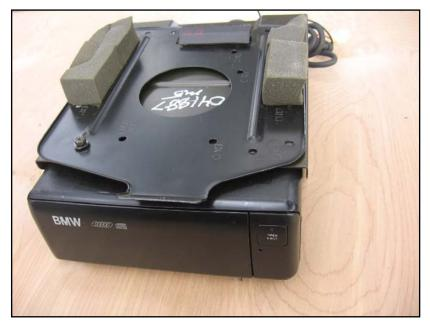
Wide tab at center rear of the top plate fits into a slot on the uppermost plate that is shown in a picture below.
