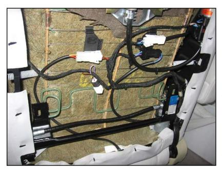
Attach the seatback. Plug in and zip tie the seatback connectors and harness once the seat is assembled in the car (see seat heating chapter for some zip-tie locations).
