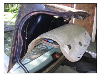
The tool box and the four screws along its bottom edge do not need to be removed to allow access to the wiring path, though the box needs to be opened up. Note existing harness, held in by a white clip and wrapped in black friction tape, at left of the trunk lid.
