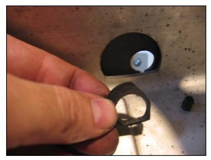
Beveled washer cut to fit along the edge of the bumper carrier pre-cut hole. You shouldn't need to do this if you use the revised method described in the text earlier, for later cars.
