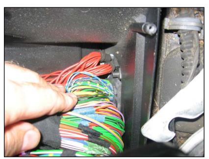
Find where the wires go from the very bottom of the front fuse box through the firewall into the underdash area.
