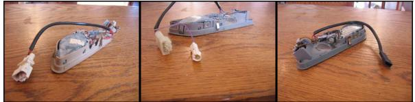
Early, mid, and late dual rear interior light units showing the different wiring connectors.
