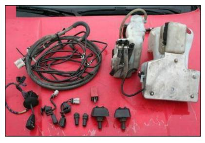
A headlight and intensive wash system – fluid hoses, tanks, wiper stalk, heated windshield nozzles, fog-light nozzles, control module, and headlight nozzles. Note that these tanks are not for the E34.
