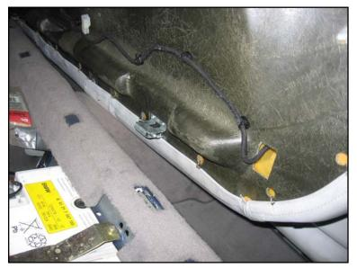
Finally, connect the connector to the rear headrest switch and install the switch into the trim piece. I found it easiest to install the switch first, then maneuver the connector into position through the access hole and lever it on.
