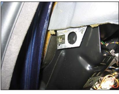
Remove small plastic trim-colored cap at side of trim, and remove screw that goes into this speednut.
