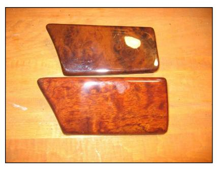
Right-side wood trim, glove box version at the top. It's hard to see in the photo, but the glove box piece has a warped shape, unlike the original. The lower piece looks bigger only because it's closer to the camera; the very slight difference in the angle on the left of each piece is real, however.
