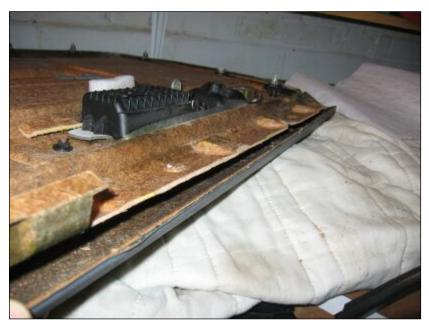
Put the main roller in place, and mark where to cut away a long slot for the shade to come through near the top of the door panel. The cut must be made without cutting into the topmost layer of the door panel (see more on the topmost layer, below). The fiberboard can be cut carefully with a reciprocating saw, or more safely and much more slowly with a sharp hobby knife. The fiberboard cuts relatively easily with a knife but requires numerous passes.
