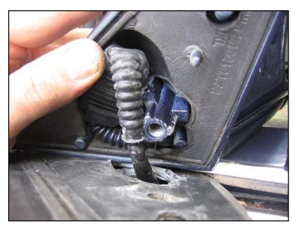
Mirror harness connectors scrunched into their cut-out in the mirror foam spacer on the passenger side.
