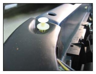
Upper plastic rivet. Pin is pulled out part way to release rivet.
