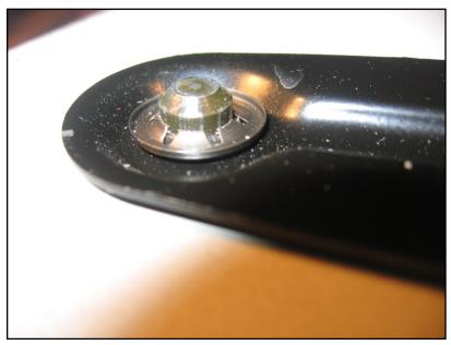
The EBA says that the armrest is attached to the old bracket with a bolt, but in my case it was a one-way toothed spring clip, which was somewhat hard to get off. Lever it up gingerly, perhaps with a pick under the teeth, and preferably buy replacement clips ahead of time in case of breakage.
