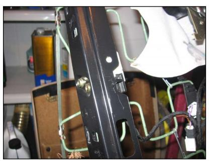
My donor seat used a relay, bolted to the seatback frame (like the headrest motor but on the other side) that needs to be transferred along with the seatback harness. Unbolt its bracket (and put the bolts back in the bracket for now, so you remember which ones they are).
