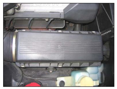
Remove the air filter box, in order to be able to remove the plastic trim behind the right headlights. When lifting out the box, be aware that the rubber mounts underneath might fall off the box onto the ground or the engine-bay pan.
