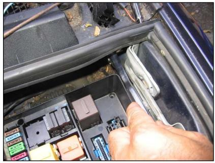
Unbolt the hood guide and move it out of the way.
