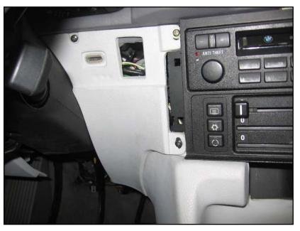
Screw on the right-side trim – one screw at top left, two screws on center console.
