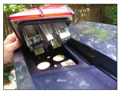
Crimp another contact to the end of the additional wire, secure it along the existing harness (there are access holes to reach inside the trunk lid shell), and insert it in the right-side connector (**X328/3**). The new light assemblies will handle ground through a pre-existing common ground.
