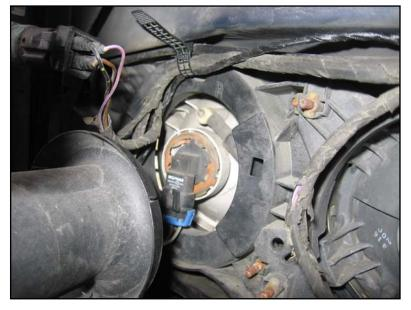
Secure the wiring anywhere else needed.
