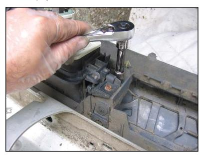
Take the protective strips off the top of the bumper (see picture later of removed bumper cover).
