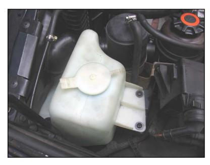
Insert the plastic nuts into the square holes in their flange near where the top of the tank goes. Insert the tank into the locating slot at the bottom, and screw it down.
