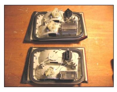
European version for fog lights at top. On the U.S. version, note the fog-light area, which has the raised surface for the bulb holder, but no pre-cut hole (or even cut lines).
