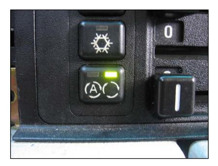
Alright, that's it! Now, when driving along with the controls in auto mode, you should, when stuck behind that smoke-spewing industrial truck, be able to hear your vents closing, without you lifting a finger ....
