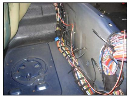
Lay wiring harness alongside the large existing wiring loom covered by the channels, and lay the relevant branches up towards the headrest brackets, past the seatbelt latches.
