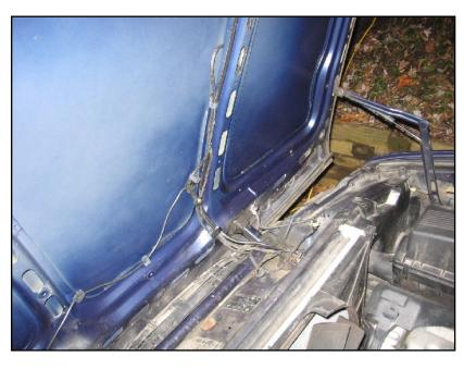
Lower routing. Wire to the hood switch is going to the lower left.
