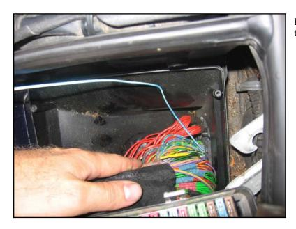
Ease a new wire through the hole into the under-dash area.
