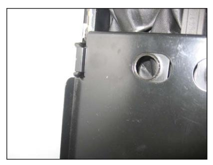
Close-up of bracket in place with latch (out of view on back of bracket) engaged over brace on seatback.
