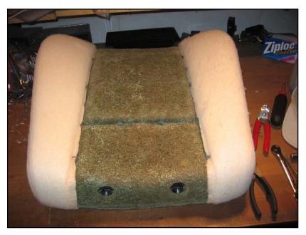
The seatback with the cover removed showing the fiber support mat in the center.
