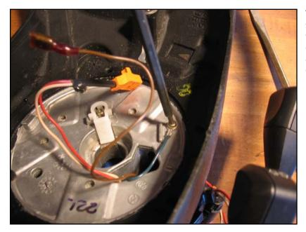
Take off the donor airbag if any, remove the wheel from the column, then undo three T10 Torx screws on the back of the wheel, and another one holding on a blue wire on the front of the wheel.
