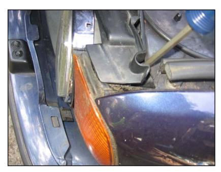
It's difficult to get the screwdriver in the right place at the bottom through the small hole, unless you pull off the headlight rear trim, and look for the small round hole on the sheet metal. It is very hard to spot the hole, the headlight assemblies are in the way, but it is possible from certain angles. Guide the tip of the screwdriver through that hole.
