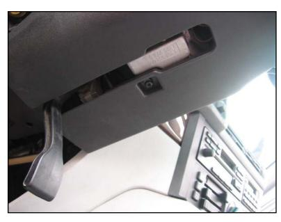
Screw-clip on the lower steering column cover.
