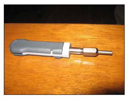
The light-gray plastic part slides up over the end of the tool when it's not in use, to protect the tool tip.
