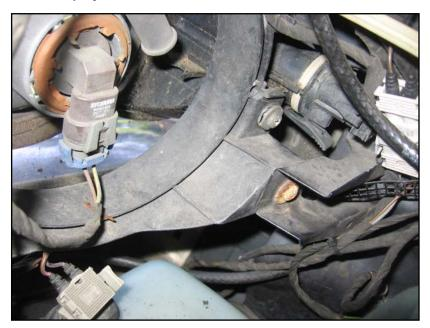
Finally, remove three screws at the outer side of the rear of the headlight assemblies. These screws are hard to reach – remove the trims behind the headlights for easier access.
