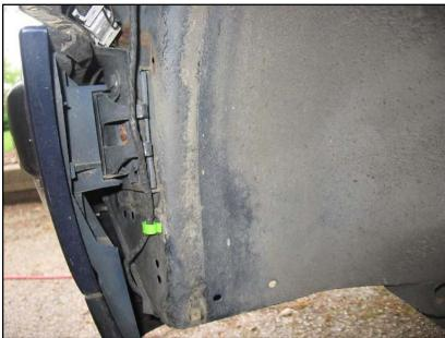
Exactly where the harness was intended to run into the engine bay was not clear. You can go low and under all the sheetmetal, or high, past the side-marker light area. The high route would seem normal, but there was a surprising amount of slack in the harness when using that route.
