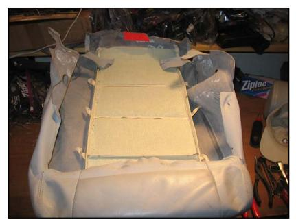
The inside of the seatback cover, showing the long sleeves along the seams that hold the rods for the hog rings.
