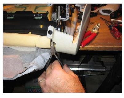
Push-clip on rear of trim – you can squeeze from the inside as shown while prying out from the front.
