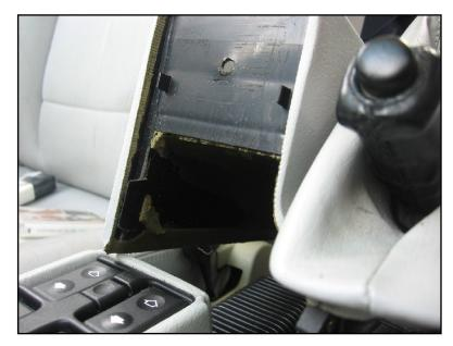
Rear console released. Slide out large securing tabs, for example the hard-to-see one on the console's lower right edge.
