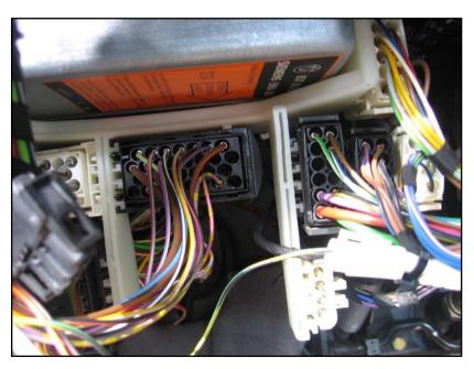
Unfortunately the large white connector carrier at top left of the driver's footwell only has the attachment points for wire connectors, not the ones for relay holders. (There are adapters on the car that will allow a wire connector or fuse holder to be put on the relay attachment point, but not vice versa, that I've found.) Use hookand-loop material to stick the relay holder or the control module to the side of the white connector carrier, the SRS module, or a similar spot.
