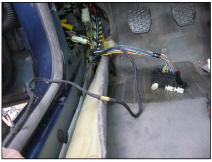
Lay the appropriate branch of the harness forward to the left door connector (shorter branch to **bk** 10-pin) and to the steering column (if an appropriate white connector is included on the harness for the optional electrically-adjustable steering column).
