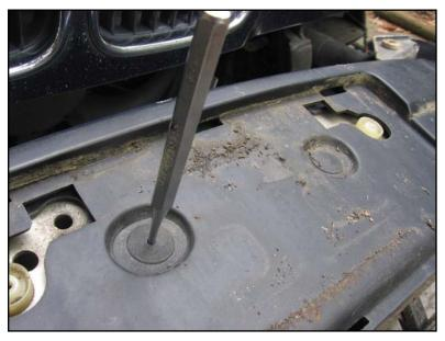
Remove the center trim by pushing in the plastic rivet pins (don't damage them, so that they can be re-used) and levering out the retaining lugs.
