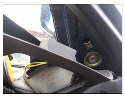
Take off the screw holding on the speaker trim to gain good access to the single bolt holding on the mirror. Unbolt the mirror (6mm allen wrench) while holding it from the outside.
