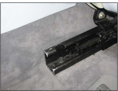
Move the seat forward so the seat bolts at the rear of the seat rails are exposed. If you're lucky, your donor car still has power (make sure there's a fuse in F16 or F18); if not, the factory thoughtfully put in a power-failure backup capability: the front-back movement motor can be turned manually.
