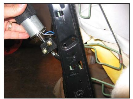
The headrest motor simply unbolts from the side frame.
