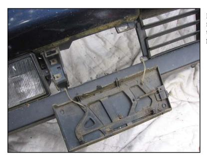
Remove rectangular trims next to the fog lights by sliding in the spring-loaded tabs. The trims are likely to be stuck in place by grime.
