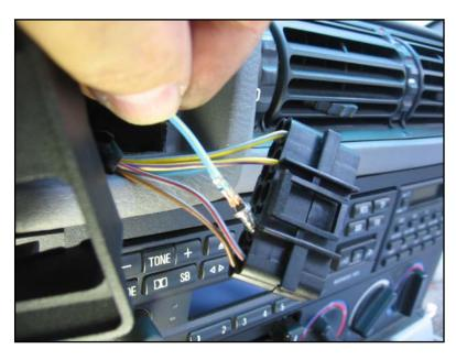
Feed a wire (I used 1 mm²) up the left side of the footwell, and up behind where the instrument cluster normally sits, toward the switch location. Bring the wire out through the switch hole. Leave slack for now, until the next few steps are done.
