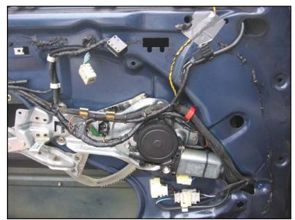
of the supplementary harness, and test fit the panel as necessary. Make sure the new wires will not ever stray in the path of the toothed regulator section visible in the picture, or other moving window parts. Run the window up and down, while being ready to halt it quickly if needed, to see the wide area the toothed piece and other parts travel in.
