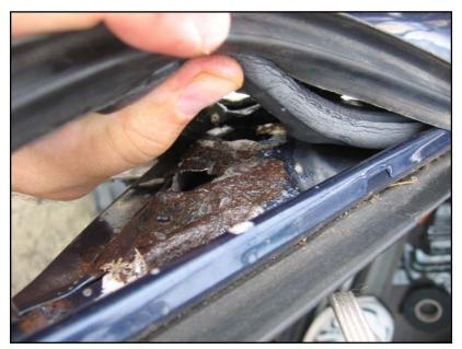
Lift away the door weatherstrip and foam packing pieces to see the full extent of any damage.
