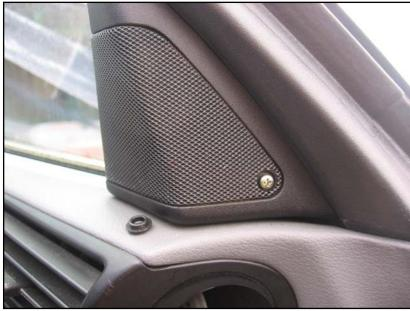
Pop off the screw cover and take out the screw holding the door speaker grill and speaker.
