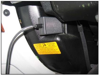
Power adapter plugs into flashlight-charging socket behind glove-box door. Note the clear reinforcing plastic on the cord that helps protect the wire when the glovebox door is closed over it.
