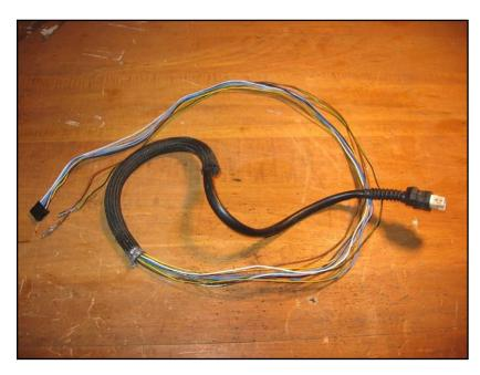
Perform a similar operation for the passenger door harness. The passenger harness has fewer splices, and the relevant wires can be liberated without any wire cutting.
