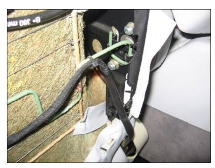
The picture shows a close-up of the bracket that supports the right side of the adjustable lumbar support. Remove the green rod by loosening the metal flanges holding it in at left and right, and cut the wire tie visible in the picture.
