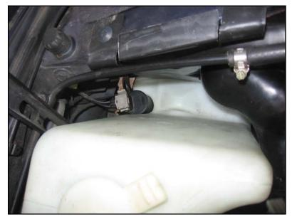
Attach wire connector to pump.
