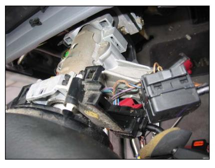
Squeeze the tabs to release the wiper switch and stalk.
