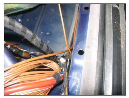
On the right side, the ground wire from a donor E32 may go forward into the wire channel along the right rear passenger door sill to a dead-end splice, then double back to the ground point in the right rear seatwell.
