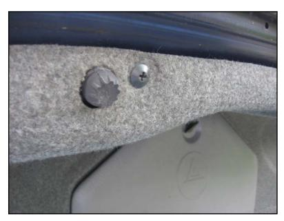
Take off the trunk lid trim to access the light assemblies. There are four turn-release clips at the bottom edge (i.e., when the trunk lid is down) of the lid, and all the rest just pull out.
