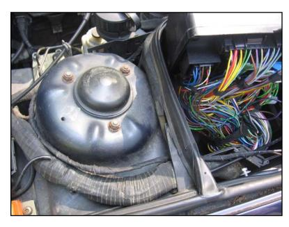
Finally, loosen the cover on the front fuse box wire-entry hole and put the harness into the box, and then through the grommets into the inner chamber. A cable strap holds the big harness by the strut tower (not present in this picture); if it or others break, replacement cable straps are 61 13 1 389 024 or 61 13 1 373 565 (shorter).
