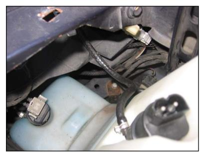
Run the hose to the intensive pump, clamp it on, and insert the pump into the tank through its grommet.
