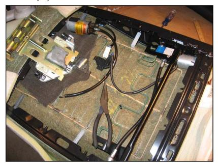
Clip on the connector holder, very gently (the thin lattice-wire-gripping tabs can be extremely brittle), and zip tie the cable to one of the lattice wires.
