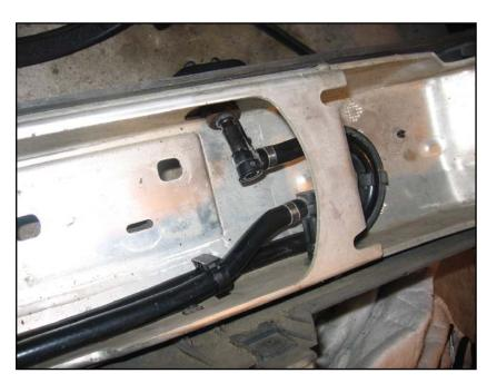
Right-side hoses attached, with cshaped hose brace visible at right behind the metal bar.
