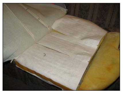
Unlike the seat heating elements for the front seats, the rear elements I ordered did not come with a cut-out to go around the hog rings on the lateral metal rods. The heating wires, however, were clearly placed away from the rods and rings, so I cut slits that allowed most of the rings to be attached.
