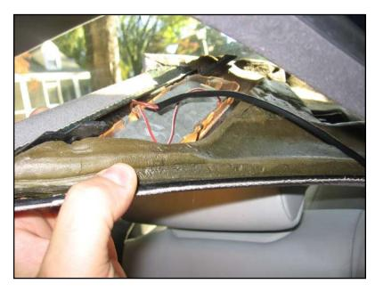
Take off the c-pillar panels by pulling straight out at the corners, in order to slide the tabs on the panel out of clamping clips in the pillar.
