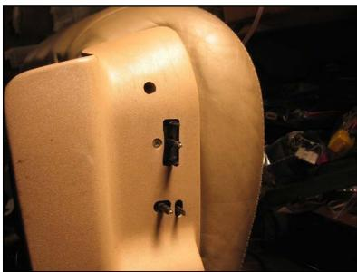
Gently pop off the seat position switch knobs, and unscrew the one, or two, screws holding the switch to the trim.
