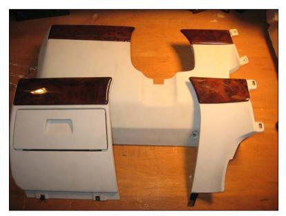
U.S. cars have a single trim panel that covers both sides of the steering wheel, but the European cars have two (in some early cases the center console piece simply extends further to the left over the right panel area), leaving the area underneath the steering column somewhat uncovered. The European cars had a longer lower–steering column trim piece that covered the gap.
