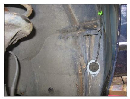
Install the large harness grommet into the hole.
