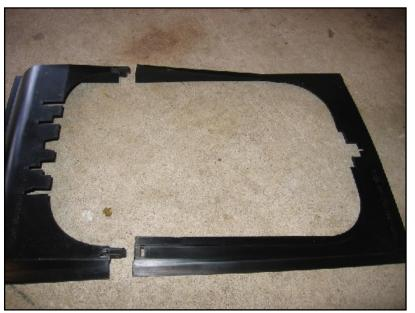
Step 4. Attach frame to ski sack and install on bulkhead
