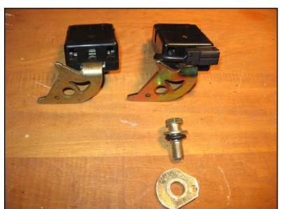
Motor connector-securing clip.
