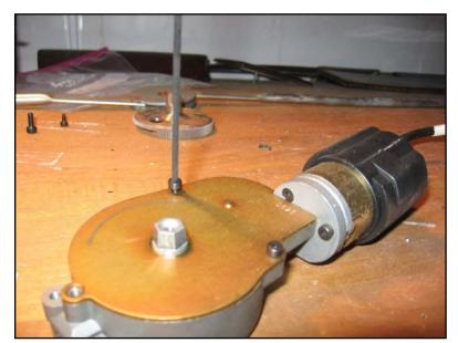
The gearspring in the gearbox is under tension and is fairly strong, so wear eye protection, and in the next step hold down the main wheel and the spring underneath it so that they don't fly up: remove the three bolts (2.5mm allen) while holding on the cover of the gearbox, and gently lever off the cover while holding the main gear in place.
