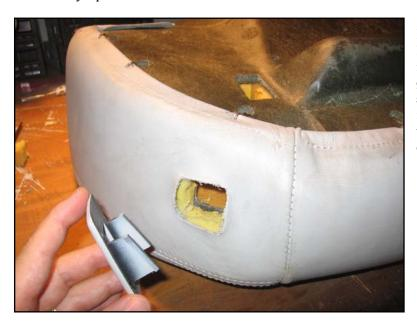
Install the switch trim piece, latching its hook ridges over the stiff black seat material – hook one side over, then gently but firmly push the trim sideways until the other side can be inserted. Don't break the trim. It's a tight fit, which is good so that the trim doesn't pop out later on.
