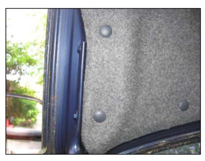
Majority of the clips are these difficult press-clips. It's hard to get them out without damaging them. One trick is to pull them and the surrounding trim material out far enough to slip a screwdriver behind the material and into the slots in the prong of the clip, then pry out gently from there—the teeth will be slightly damaged, but not too much. Clips at the bottom right of the trim material, when the trunk lid is up, should not need to be removed at all.
