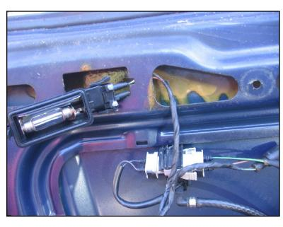
Light ready to be inserted into its hole. Securing tab is on the left, push light assembly left to release when removing from hole.
