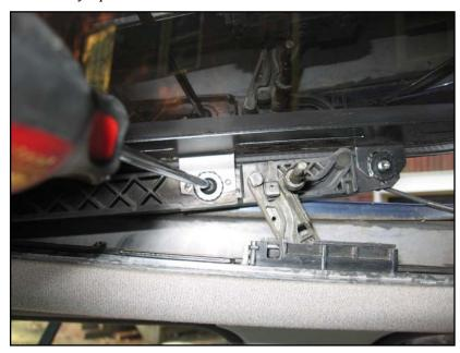
Move the sunroof forward again. Unscrew the three bolts (T25 Torx) now visible on each side.
