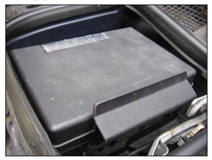
Starting with the power end of the circuit, open up the main fuse and relay box (hereafter, "front fuse box") in the engine bay.
