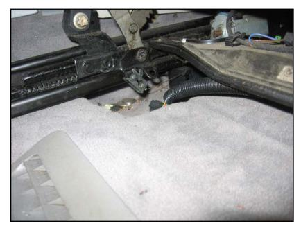
Look on the left underside of the seat for a thin bare wire running back to an articulated metal piece at the rear of the seat base. If the donor car is soon to depart this world and be recycled, just cut the wire; otherwise you can disconnect it: the wire is held in place with a pin that can be pulled out of the metal piece at the rear.
