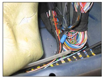
Splice the other end of the lighting power wire to one of the other small **gy/bk** wires along the left door sill (that color wire is usually an interior illumination wire; check it before using it – 12V at the end of your wire when the light switch is on).
