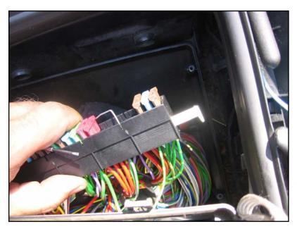
Look at the top of the fuse slot and locate the square holes on either side of the middle of the correct contact. Then push a fuse contact—releasing special tool, or more likely, if you don't have it, micro-screwdrivers, down the holes to move inwards the slightly-bent tabs that hold in the contact. When both tabs are moved, they will clear the flanges on the holder and the contact can slide out.
