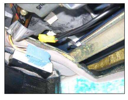
Remove the sunroof switch panel – several tabs at the sides and rear. Look for the tied-back harness in a plastic sheath with a three-pin, depending on the year, connector and free it.
