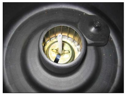
Close up of the spare wheel holder held in place with a wing nut, viewed through the center of the storage tray. At top right is the wheel center-cap remover, which doubles as a trunk-floor support when it is put on the spare tire bolt.
