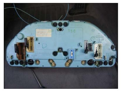
Now prepare the wire going to the "rear fog light on" information light on the instrument cluster. This short wire will go from the back of the instrument cluster to the main wire that leads rearwards to the rear fuse box (see earlier diagram of circuit).
