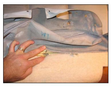
The seat base has two rods going left-toright along the seams, and the seatback has one. The rods are clipped with hog rings to matching rods inside the seat foam (for the seat base) or to the underlying support mat (for the seatback – the mat is made of glued-together strands of some kind of fibers). Whereas the originallyequipped elements go under these rods, the new elements go between and partly over these rods.
