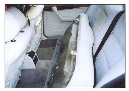
There are some strong steel bar springs that hold the seat down, and the pulling must pinch the springs inward to let them pass through the slots they're in. The accompanying picture shows the two brackets holding the springs – the springs stick out left and right from the brackets.
