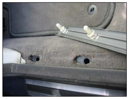
Lift up rear passenger footwell carpet to access the wire channels. The carpet can usually be slid out from under the sill trims and b-pillar trims, but if desired the trims can be removed first. Lever them out firmly. Removing the front seats can help to pull back the carpet more easily, but it is not necessary. If removed, the seat bolt torque is 44 N-m, for reinstallation.
