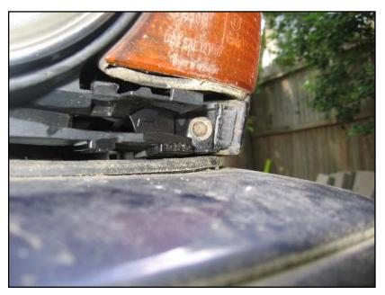
Single screw underneath the turn signal.
