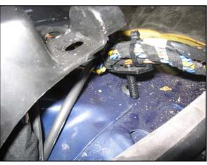
Thick wire-securing pins at front top left and right of seatwell pull out of rubber grommets.
