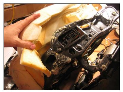
The seat foam can be left on the seat frame, although it might make it marginally easier while you're learning how to attach the hog rings to be able to bend back the foam while it is off the frame. If so, the seat base side bolster foam may have some rubbery glue holding it onto the frame – peel the foam back carefully so it stays intact, and re-glue it if desired when reassembling.
