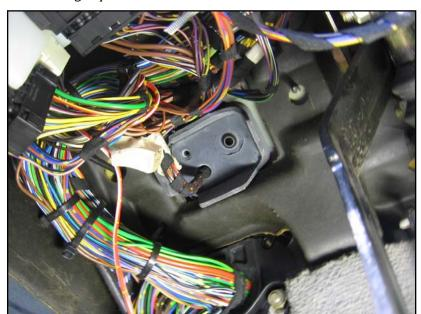
Wire 3. Splice a wire from the Raintronic module terminal 31b to the **br/gn/ye** wire already going to the wiper limit switch in the wiper motor. There are no junction connectors for this wire in the under-dash area, the wire goes directly from the General Module to the wiper motor, so splice in to the **br/gn/ye** at a place like this.
