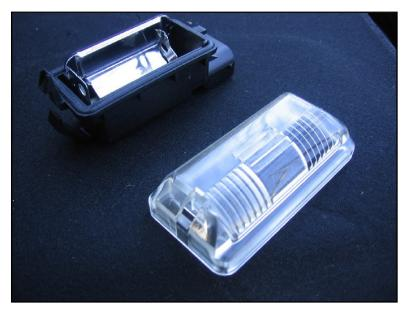
**Step 3. – Install components**Connect the rear half of the light assembly to the wiring harness and insert it in its hole in the hood – connector to the right.
