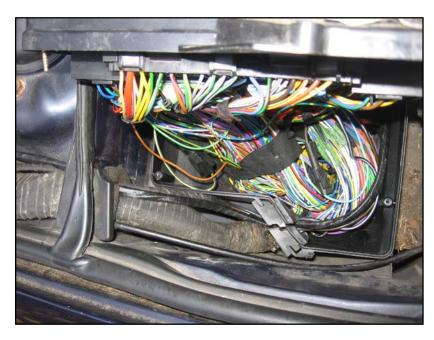
Run the harness into the waterproof area through the hole, then into the fuse box itself through its grommet.
