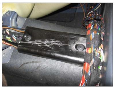
Pull back the carpet over the transmission tunnel, and unscrew the thick wire channel that lies along the top.
