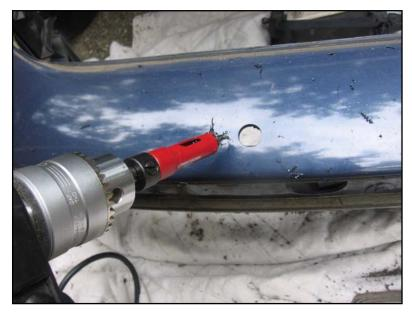
Then drill a pilot hole through from underside to top side, as for the fognozzle hole, and drill the 16mm hole from top side to underside (using a hole saw with a pilot bit, I found no need for the 3.5mm pilot hole described in the EBA).
