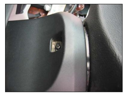
Take off the upper steering column cover – one screw-clip on the top, locking pins connecting to the bottom half, and one screw-clip on underneath. This helps for removing the cluster completely. The upper and lower halves are quite tightly connected together: pull firmly but carefully so as to not break the locking pins.
