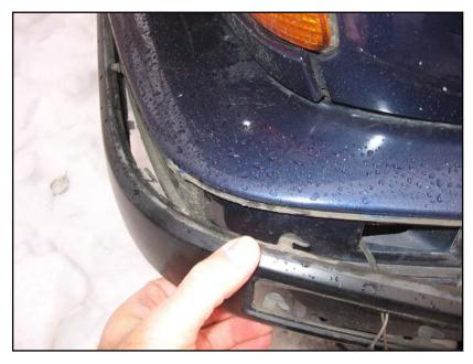
Note the hook on the tab on the side of the trim (bottom right of the picture). Several of these hooks on the trim along the side of the car need to be slid forward in their slots, then the trim can be pulled out laterally. The trims are often crusted in place with dirt, and hard to slide. Note the wires and hole in the sheet metal for the light assembly, at the bottom right of the picture.
