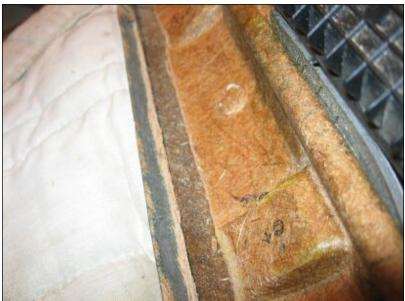
Covering (grey material to the left) carefully cut away from fiberboard (next strip to the right), and fiberboard removed.
