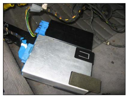
If you have cruise, it seems that the cruise control module bracket is also designed to hold the AUC module. One side of the AUC module bracket slips into a slot in the cruise bracket behind the cruise module, and the other side needs a plastic nut on a bracket stud.
