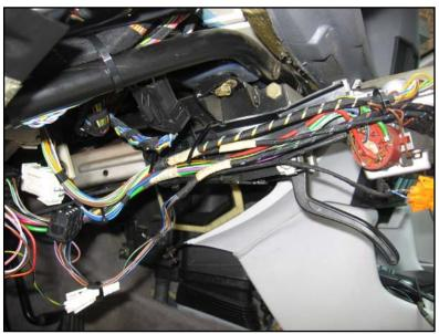
Remove the steering column trims (see chapter on rear fog lights).
