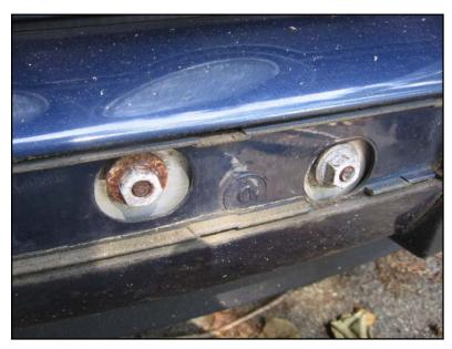
Unbolt the bumper. (It was a very tight fit to get the bumper back on those bolts during re-installation – it looked like the bolts wouldn't fit into their holes, but they did, with some force and maneuvering. Try levering the bumper over the bolts with a screwdriver, if necessary.)
