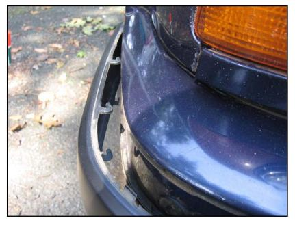
Lever out the black plastic side bumper strips, starting from near the license plate. Once the clips on the front side are free, just slide the whole strip directly forward about a half inch, then the hook-shaped clips on the side should be free and you can pull the strip out to the side.
