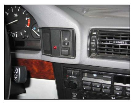
Alarm LED relocated from rear of center console using wiring kit (microphone is not yet in place just above the LED).
