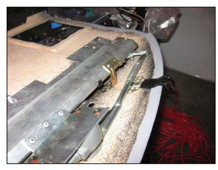
The gold-colored brace towards the center of the picture is one of three that position the rear of the parcel shelf relative to the shade mechanism.
