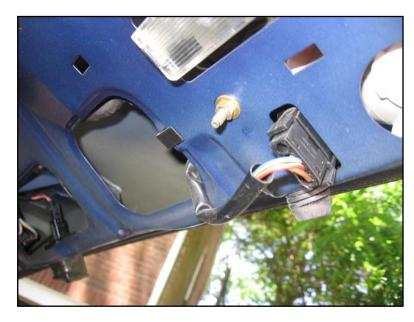
Note the black harness clip near where the wire harness goes in the trunk-lid hole. The additional wire can be inserted into such clips.
