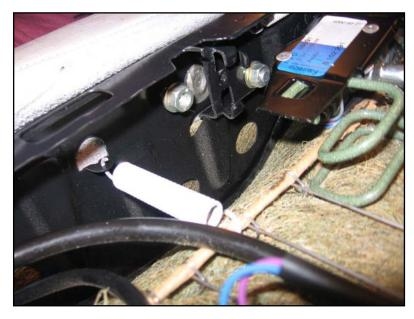
Remove the armrests by taking off two nuts inside the seatback frame.
