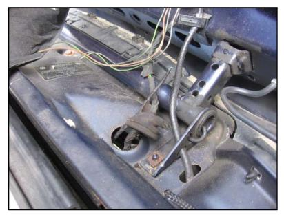
Then pull out the upper grommet and fish the new wire up through the hole.
