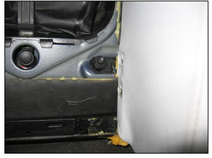
To remove the seatback, start by unscrewing the nuts behind the center armrest.
