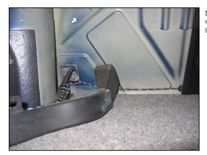
Now you can see where the harnesses come into the trunk through the rubber grommet in the bulkhead.
