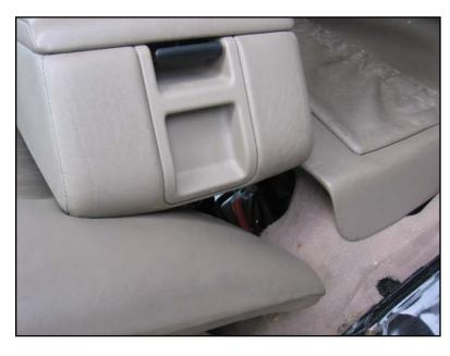
The late-type armrest is also distinguishable by having only one release button on its front. That button releases the compartment lid; unlike for the first armrest, there is no button to lock the armrest in place, up or down.
