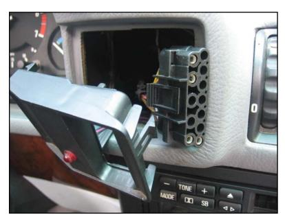
Gently lever out the fog-light-switch trim, remove the old switch by pushing it out the front of the trim, and disconnect the connector.
