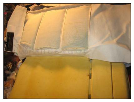
As for the front seats, cut slits in the fleece on the undersides of the covers, and slide in the elements. You may need to cut another small hole for the wires, which come out at the front end. Stick adhesive areas to the covers, then reinstall the covers.
