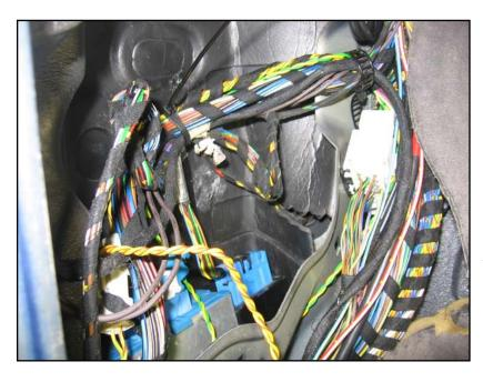
If not already done, connect the AUC control module connector: pull up the black slide lock on the middle of the connector, plug in the connector, then slide down the lock.
