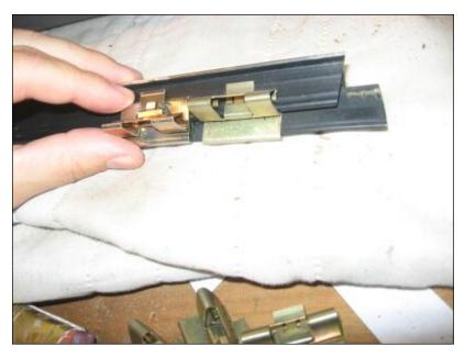
Compare the old and new clips and note how the new ones are intended to hold a somewhat deeper vertical strip, which is now going to be the side of the roller, soon to be located where the door fiberboard and its vertical strip will be cut away.
