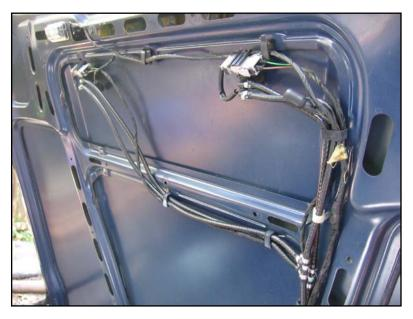
Lay out and secure the new hoses in the existing hose holders on the hood. Run the hose down through the hole in the horizontal sheet metal in front of the radiator, toward the tank.
