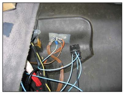
Crimp a relay contact onto a long wire that will go to the left rear light cluster (measure how long and cut to that length) and insert it into the terminal 87 slot on the relay connector.
