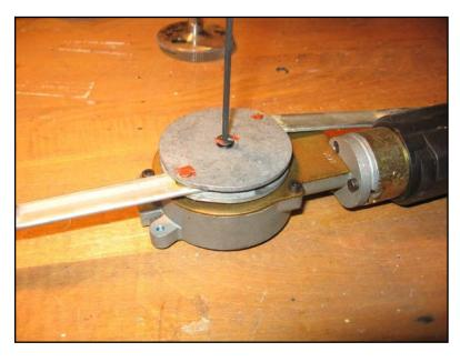
Unscrew the bolt holding the crank arm wheel (2.5mm allen) and remove the wheel and crank arms.
