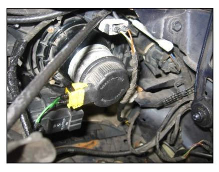
On the right side, if you're using the side-marker circuit to power the underhood light, do a splice in the power wire leading to the citylight connector to power the underhood light too.
