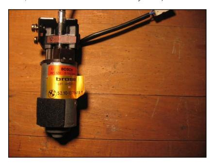
Headrest motor with potentiometer (black device at the top). The motor itself is the same for memory or non-memory; memory simply adds the potentiometer.
