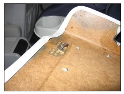
Seatback trim. This is a view of the bottom right corner, looking to the right. Pull the trim up and out at the bottom to lift the spring clip shown off the edge it grips.
