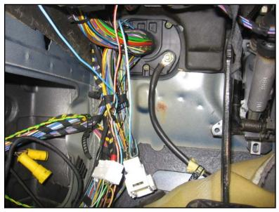
Pull the wire through and down to **X13**, a large white connector clipped to the lower left side of the footwell.
