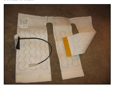
When seats come from the factory with heating, the elements are permanently attached, sandwiched between the leather and a sewn-on fleece and cloth layer. Fortunately the replacement elements are made to fit without having to sew them in.
