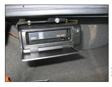
Door flips down, so this is a Pioneer. Six-disc magazine is visible inside the changer.
