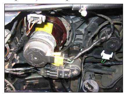
View of the left side with all connectors connected: top left, grey: city-lights; right, white: high-beam; bottom, black: headlight motor; center, yellow: low-beam.
