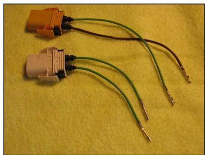
If using the European headlights, new wire connectors will be needed since the European headlights use the standard factory connectors, while the U.S. headlights use completely different ones.
