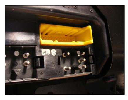
Connect the other three connectors on the supplementary harness to these slots at the rear underside of the memory control module.
