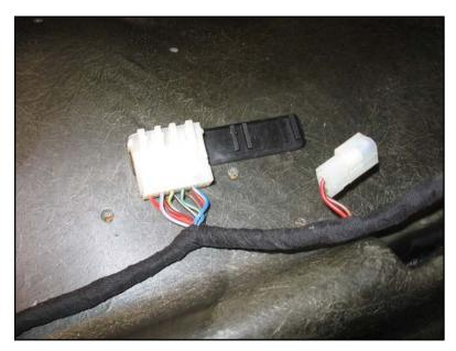
• finally, connect the main harness to the seat base harness.
