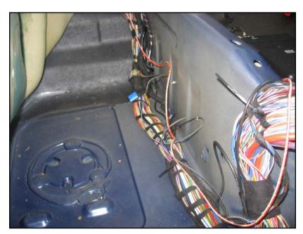
Lay the wiring harness alongside the large existing wiring loom.
