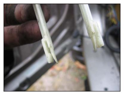
Then pry up both the bottom ends of the clip to ease it up off the box.
