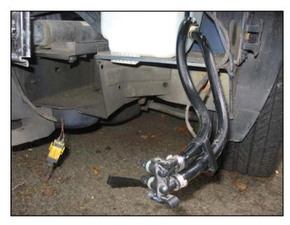
If not using an already-assembled system, connect hoses to the tank pump and the connector for the distribution block. Put a hose holder around the hoses 200mm from the connector. In the case of the 535i, run the top pump hose forward to the **top** distribution block port. Other models can run to the bottom port.
