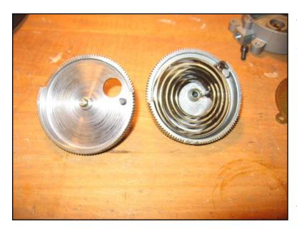
The correct orientation of the spring in my case is shown in the picture: the spring should *compress* when the wheel rotates *clockwise* when looking down on the wheel in its gearbox.
