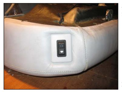
The solid white arrow on the switch points up when the seat is in the car. <sup>36</sup>
