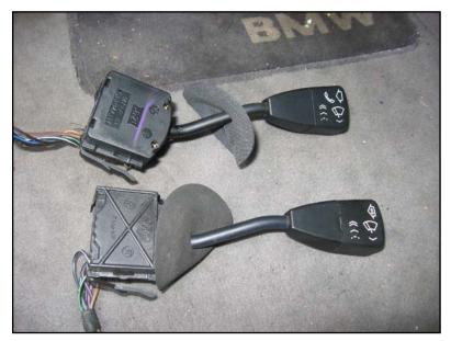
The intensive pump is activated by pushing the end of the lever inwards, and the relevant wires are the ones coming out of the stalk itself (see picture). On the regular switch, one of the brown stalk wires already goes to an appropriate **bk/gn** wire (leading to a single-pin connector near **X295**); the other brown wire might need a new dedicated wire to duplicate the **bk/vi** wire of the intensive switch – check the telephone wiring diagrams.
