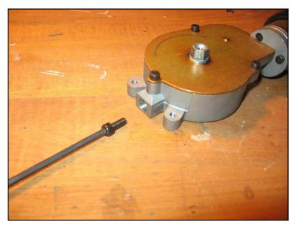
Remove the spring stop bolt (3mm allen) on the end of the circular gearbox (the spring shouldn't uncoil yet, it and the gearwheel are prevented from turning by the rest of the gears in the geartrain).
