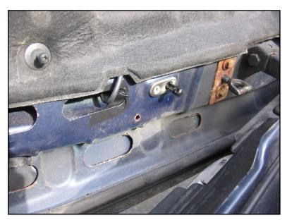
Check the underhood insulation edge near the underhood light contact switch for a slightly indented section, which indicates where the wire to the switch is intended to lie.
