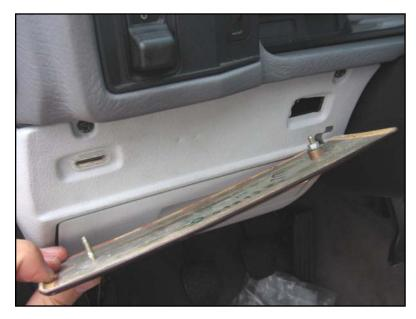
Wood trim removal: gently pry out the left side with a screwdriver inserted behind. Right side brace slides out when trim is pulled out to the left and forward.
