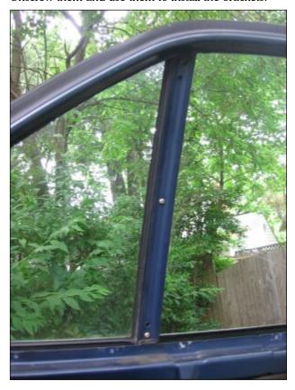
Preinstalled screws to hold on the quarter shade. Middle screw is not used, top one is hard to see in this picture, it is above the barely-visible drilled hole toward the top of the door.
