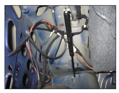
While you're there, check the condition of the wiring where it bends around the hinge: there are quite a few reports of chafing or splits in this area, leading to wiring short circuits and electrical anomalies.
