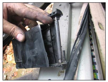
The box has two halves that clip together along the long dimension; see if you can separate them, and then see if you can push/pull a half out the front of the door. If either is negative, you'll probably have to break the box: I didn't see an easy way for the larger connectors from inside the door to get past the fixed roller bars at the front of the box (in which the rubber sheath normally rolls as the door is opened and closed). The E34 does not use this box or the sheath.
