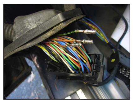
Insert the loose wire of the same **gn/bk** colors from the supplementary door harness (that we just brought through the rubber tube) into hole 18 and make sure the connector pin (female) snaps into place.<sup>31</sup>
