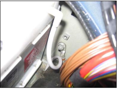
The ground point used here is on the inside front wall of the seatwell, next to the battery. Other ground points are nearby.
