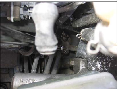
Technically, the EBA takes the column apart at the universal joint in the engine bay between the firewall and the steering rack, but the connection there was very tight and I found that method unnecessary. But to release the joint, undo the clamp bolt, and perhaps try to pry open the clamp a bit if needed to free up the splines.
