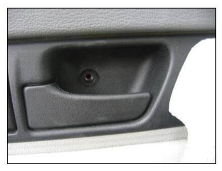
Screwhole behind door-opening handle (screw has been removed).
