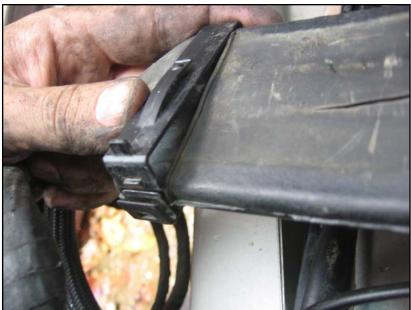
Disconnect the connectors by the door handle (three), door lock actuator, and regulator, and navigate their wires past the inner door obstructions so they can be pulled out of the front of the door.
