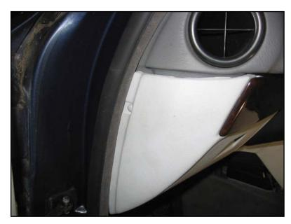
Where the new left trim panel meets the left side of the dash wasn't absolutely perfect on my installation, probably because the European dash piece is different. The trim plastic was not neat along the join, but the door is normally closed over that area, and it wasn't particularly noticeable in the first place.
