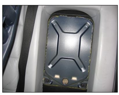
The EBA calls for painting any bare metal with zinc-based anti-corrosion paint. Spray cans of it are available to the regular consumer at hardware stores and online – a little can be sprayed in a cup to liquefy it, then painted on with a brush if that's easier.
