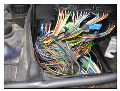
Attach the other half of the single-pin connector to the wire brought forward from **X13**, and connect the halves.
