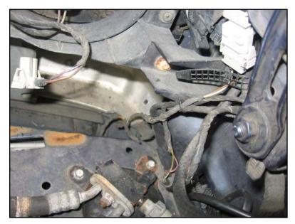
Wrap the new wire in friction tape and lay it along its path from the area in front of the windshield washer tank toward the centerline of the car. You can often feed the wire through existing wire straps without undoing them, but if needed you can carefully open them up to add the new wire.
