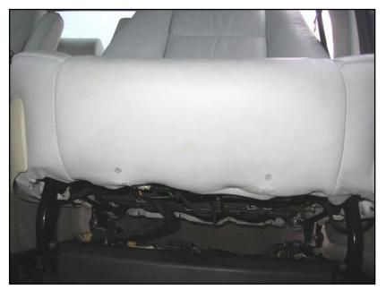
To make the incisions for the bracket and bolts, you can feel for the respective holes in the seat metal through or underneath the leather, then make a small cut and widen it in the appropriate direction. A probe or scribe can be used to locate the circular bolt holes, too.
