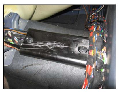
Take off the rear portion of the center console between the front seats (see chapter on electric sunshade). Pull back the carpet over the transmission tunnel, and unscrew the thick wire channel cover that lies along the top.
