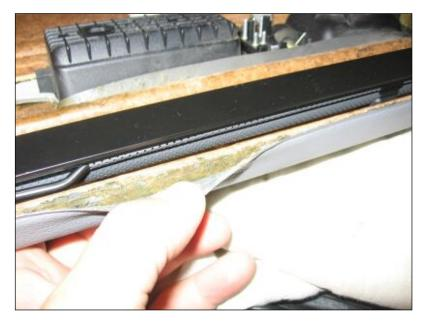
Cover plastic on top of fiberboard; both plastic and fiberboard lie atop the main fiberboard door panel.
