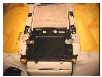
In the case of the early type of armrest, the quick-release armrest bracket just pops into place, using spring-loaded latches holding on to the braces.
