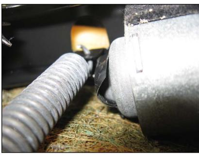
Because the potentiometer on the memory motor makes the top of the motor sit higher, it was contacting a spring on the frame in my case. I slid the spring higher on the lattice, and put some tape on to avoid potential squeaks. Consider other, more-durable solutions, too.
