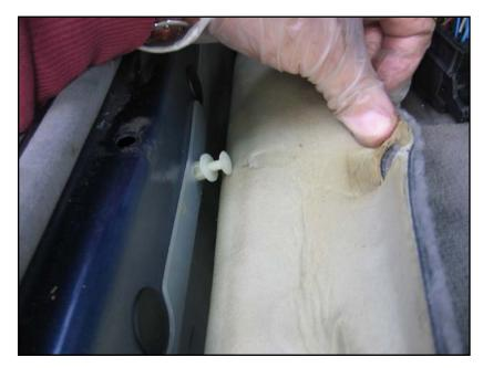
Gently pry out center pins (some may be stiff) and then remove plastic rivets to open up wire channels.
