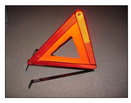
Partially-folded warning triangle, showing how the legs fold up.
