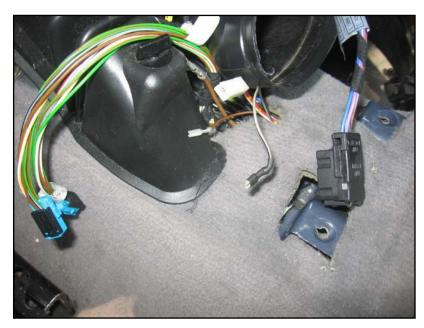
Insert the four wires under the carpet and out through the hole. Then reinstall the console and the wire channel.
