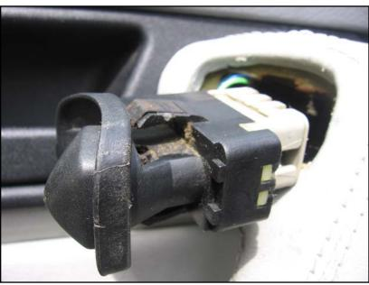
Begin by taking off the door panel and the weatherproofing sheet. Panel removal is covered in numerous sources, but steps involve removing door lock knob, cap and screw behind handle, mirror switch, and angled Phillips or Torx® screw buried behind the mirror switch hole (see above); releasing from the clamps along window; and unhooking the Bowden cable.
