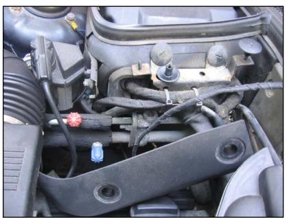
I re-wrapped the pair of wires in friction tape, which took quite a while, but was worth it for the stock look. Plug the connector onto the pump and run the wires from the intensive tank around the back of the engine bay to the front of the fuse box.
