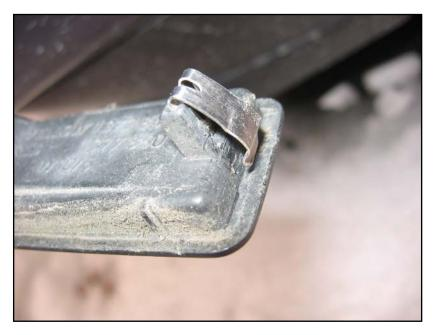
To access and disconnect the sidemarker connector, remove the sidemarker light assembly, hopefully by sliding it backward in its receptacle against a spring clip at the rear until the front tabs clear the trim and the assembly can be pivoted out. Unfortunately the spring clip system does not work very well in this application, and the assemblies often have to be levered out, bending the clip. Watch out, the clips are not attached very firmly and can drop out.
