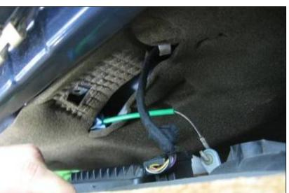
Window switch connector, shown with the door panel already off. Note also the black plastic door panel main clip below it. Remove it, and reattach it to door panel before reinstalling the panel.
