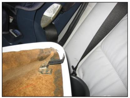
The clips shown in the picture hold the top of the trim in place. Once the bottom of the whole trim is out, push down slightly on the panel, so these top clips clear the seat frame. Be careful not to rip any of the clips off the panel, they're not strongly attached.
