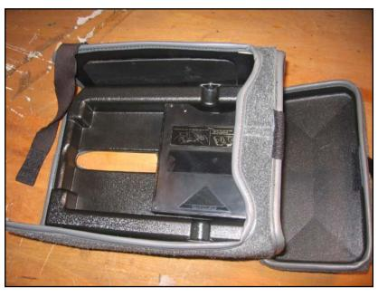
The rear of the cover is held on by the elastic strap visible in the picture. It simply goes over the top of the changer/plate and attaches with a hookand-loop patch. Note the CD magazine sitting in the tray at the bottom of the cover. Two magazines will fit in the tray. Perhaps the long hole visible in the bottom of the cover is meant for sticking in a finger to fishing out a magazine from the back of the tray when the cover is installed.
