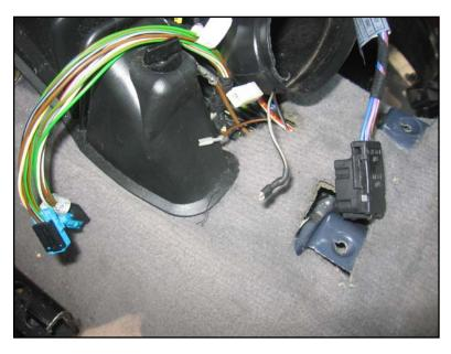
If installing the electric rear sunshade, also insert the wire leading to its switch along the same path. (Now is also a good time to put in the rear console power outlet wiring, which goes along the same route.) Then reinstall the console and the thick wire channel cover. Connect the wires to the electric headrest switch in its tray on the top of the console, and to the seat-heating switches and power-outlet socket on the back side of the console pop-out panel. Re-mount the console and panel.
