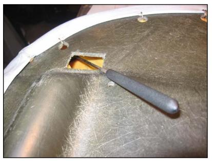
Look down into the holes and you will be able to see a corresponding hole in the same black shell along the side of the seat. Use a probe to indicate where the latter hole is, roughly, then cut out a matching hole in both the leather and the foam underneath it.
