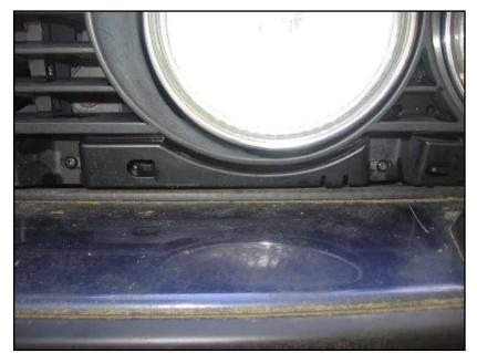
Next unscrew four screw clips and one sheet-metal screw, which hold on each side grill. They are accessed from the front. Be careful with the screw clips, the plastic screw heads can easily strip, requiring drilling out the screw.
