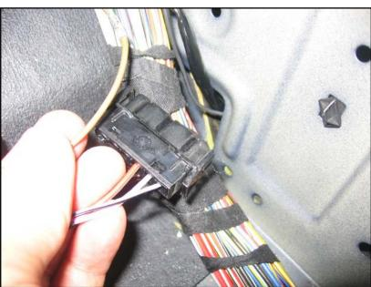
Carefully maneuver the connectors that go to the vehicle harness, seat-base harness, control module, relay, and the ground wire terminal through the small hole at the bottom of the seatwell front wall, near the transmission tunnel.
