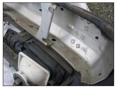
Put a pen through the pre-cut holes for the fog-light nozzles in the bottom side of the bumper, and mark the center of the hole on the inside of the plastic bumper cover (since there are angles and drawing a circle would be difficult).
