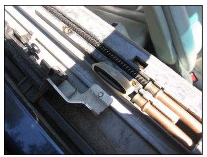
Lift out sunroof – be careful, it's heavy, and the sharp metal tabs for the screws will scratch the roof if they touch it.
