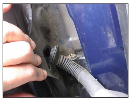
Now pull off the grommet at the door end of the rubber tube for the door harness connector.
