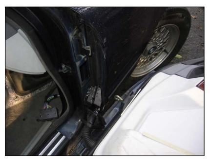
Prepare a safe place to lay the door so that the connector will easily reach its mounting hole on the body. I put it flat on an adjustable-height workshop stool, being careful afterwards not to knock it off. Then lift off the door – although it may seem stuck in the hinges, it can come off suddenly, so don't let it hit the bodywork when it does. And the door is quite heavy, so be ready for its weight.
