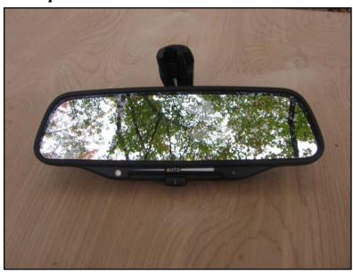
The early autodimming mirror, with slide control at the bottom.
