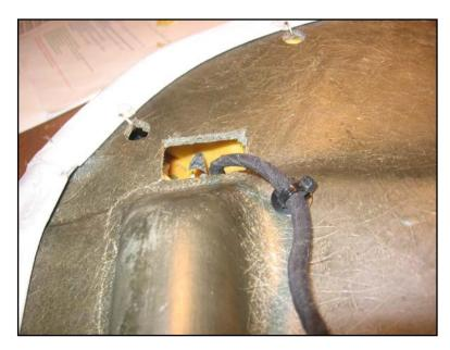
Run the switch connector on the seat base harness out to the access holes, attaching the harness by pressing the wire- and connector-holding clips into the matching pre-cut holes on the underside of the seat base.
