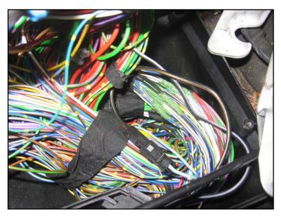
Now splice the wire from the pump to the front fuse box end of the new wire, or use a single-pin connector as I did, which works better than a butt connector if the wire sizes are different.
