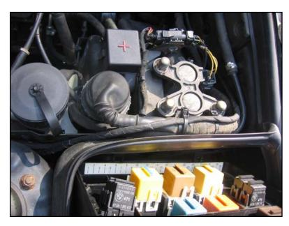
Pull off the tight cover to the auxiliary coolant pump at the left rear of the engine bay, and continue to zip tie the harness.
