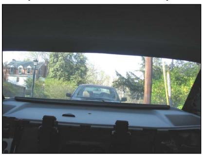
Connect the battery (run the engine if you move the shade more than a couple times so as to not run down the battery) and give it a whirl. See where and whether the shade contacts the glass, per the EBA (see above regarding the 10–15 cm specification). Note the rubber wheels on the end of the shade that let the shade roll along the window (make sure you have them!).
