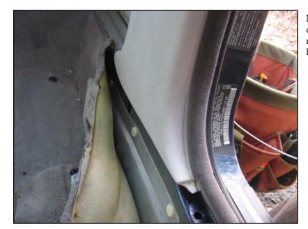
Next, remove the wire channel covers along the rear door sill and rear seat (see chapter on rear headrests).
