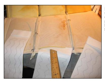
Push in the strips of the element into the appropriate sections of the cover, using a ruler in the convenient end pockets of the strips. The fleece can be loosely stuck to the underside of the leather, so clear a path first.
