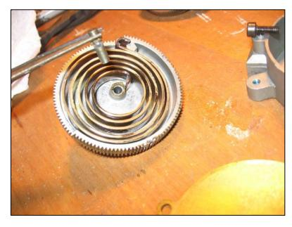
If using a new gear, transfer the axle pin to the new one.
