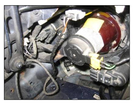
Look for the zip-ties where the foglight part of the harness splits off. Cut off and replace the zip-tie, taking up some of the slack that there is towards the fog lights, so that the city-light part of the harness will reach the city-light connector.
