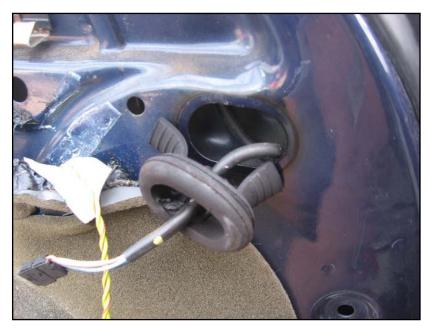
Take off the old mirror. First ease out the grommet, at the top front of the door panel, that holds the mirror harness, and push the harness through it.
