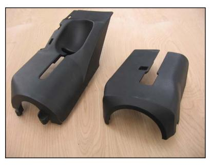
The steering column trim for driver's glove box cars extends down into the gap between the side trims. At least one such column trim did not fit on the steering column of my later car, however. Here are the different lower trims:
