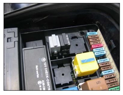
Re-insert the relay base into the front fuse box holder, from the bottom.
