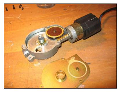
Inside the gearbox. Normally keep a hand on the large gear in case it wants to fly out. Note the spring, visible through the round hole in the large gear (shiny steel-colored). You may want to mark the rotational positions of the gears, it could be useful for reassembly, though I did not need it. Also note the axle pin in the smaller brown gear – it is nicely lubricated and can fall out.
