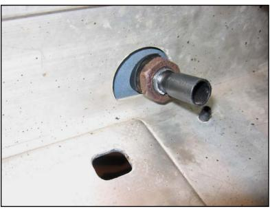
This is the headlight nozzle assembly with beveled plastic washer.
