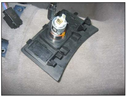
Connect the wires to the socket on the back side of the console pop-out trim panel. Remount the panel.
