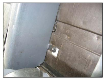
The quick-release latches on the armrest bracket hold on to braces on the seatback. On E32s, the braces were usually welded to the seatback; on the E34 the braces were screwed higher up into pre-threaded holes in the seatback.
