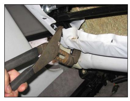
Seatback release lever being released with adjustable joint pliers. Lever can be tight, and can snap back.
