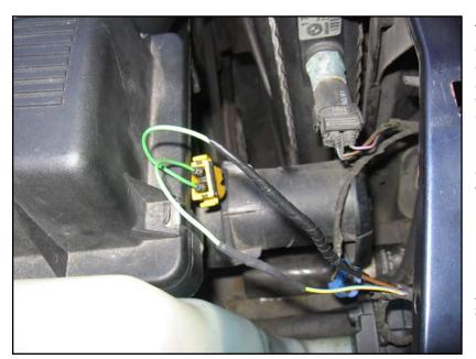
Then cut off the old headlight connectors from the vehicle wires coming to the headlights, and – always after putting on heatshrink tubing – crimp the cut wires to the free end of the butt connectors.
