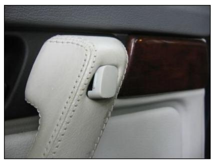
Scratchable screw cover in door pull. Note one of three retaining ridges.
