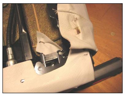
Once the lateral rods are secured except for the end hog ring, and not the left-side fore-and-aft rod, take off the adhesive cover strip and attach the element to the foam. Then re-attach the left-side rod.
