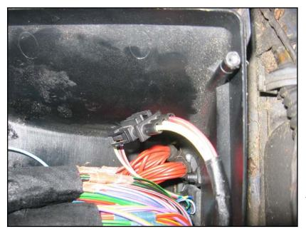
Make sure you have enough wire in the footwell (especially for the wire going all the way to the switch), then cut the wires and crimp pins on their fuse-box ends. Insert the pins in the second half of the three-pin connector, and join the connector. Don't forget to slide the relevant parts of the connector halves over slightly to lock the contacts in place.
