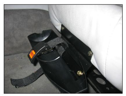
The M6x16 bolt was a little short to begin threading, so I used the M6x20s. The bolt on the left seemed to only just clear the motor behind it in the seat.
