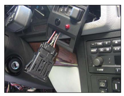
Gently lever out the switch trim, which also holds the fog-light switch and maybe the alarm sensor and LED.
