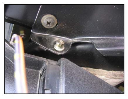
This is where the top of the left damper attached on an E32 donor car. The bushing appeared to be riveted on, so I used something similar from the hardware store.
