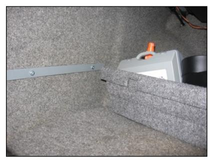
The bin is shown here dismounted from its attaching rail. The flap on the bin slips behind the rail – look closely for the rectangular cutout on the bin that goes over the screws on the rail. Bin may be thus removed completely if extra space in the trunk is needed.
