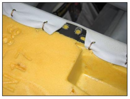
The bolt holes for the braces are precut, and the leather is somewhat so, as seen in the picture, but additional snips were needed in the leather for the latch plates to lie flush against the seatback metal.
