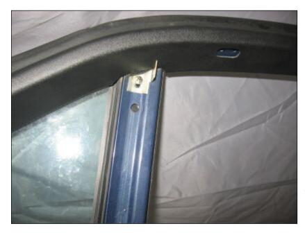
Upper bracket. Note hole in black trim for main-shade bracket screws, to upper right.
