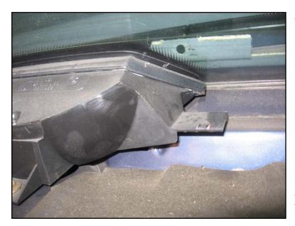
The two center clips attach to flanges on the third-brake-light housing.
