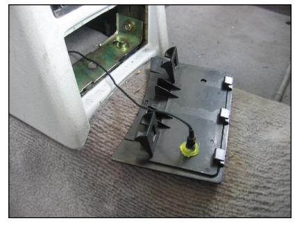
Note large tabs at the bottom of the plate. These need to be popped over a lip to release the plate.
