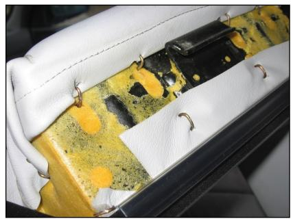
The short black metal flange, close to the top of the seatback, hooks over the metal bulkhead behind the seat.
