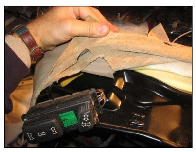
Note that the flap of leather near the seat-adjusting switch goes into the seat frame across the top of the switch hole, and hooks onto a prong pointing inwards.
