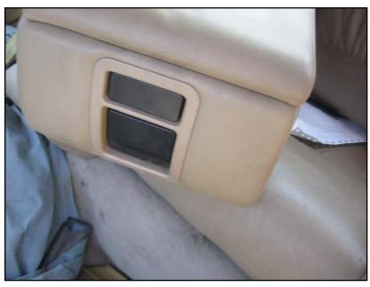
The early-type armrest was distinguishable by having *two* release buttons on the front of the armrest, one to open the lid (top button) and one to allow the armrest to be raised and lowered (bottom button). It is possible this armrest design was replaced because klutzes were pulling up or down the armrest without pushing the release button, breaking the mechanism or bending the mounting bracket.
