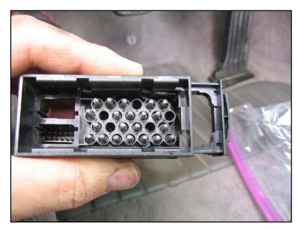
Now insert the **br/or** (mirror position switch) and **br** (mirror heater) ground wires into any free pin holes. I used holes 12 and 19.
