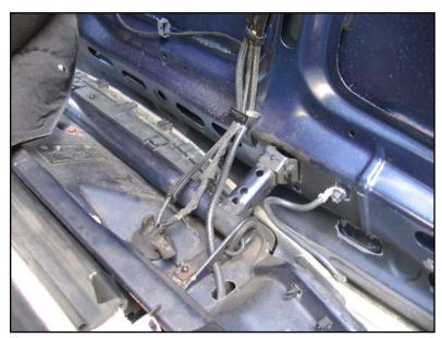
Crimp the wire to the rest of the harness on the hood. Try to put the joint in an area that gets less wet, at a minimum under the underhood insulation mat.
