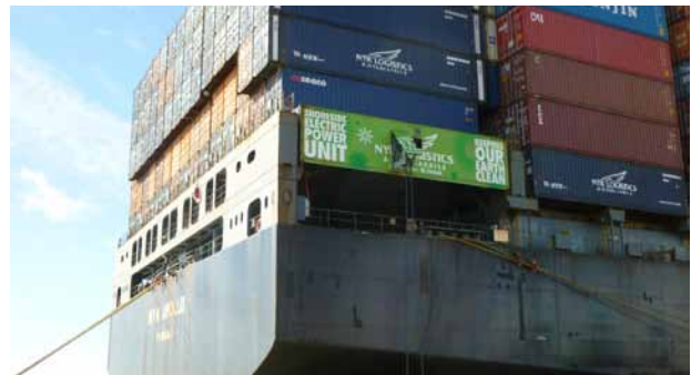
NYK Apollo connected to the onshore power supply at the Port of Oakland
