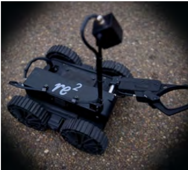
DS1-MA Manipulator Arms, developed by RE2 have been integrated onto many of the Armadillo Micro Unmanned Ground Vehicles (MUGVs).
