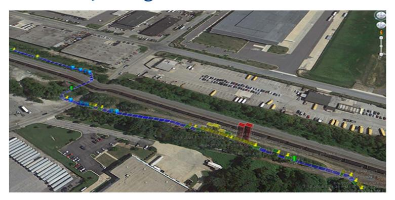
By overlaying the pipeline onto the aerial photography, we can identify critical areas such as schools, hospitals, and major road interchanges where catastrophic water main breaks can impact property, life, and safety.
