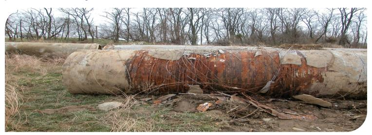
Over the next 11 Years, two leaks and five more catastrophic failures were experienced in the 36 inch Elkridge Transmission Main.
