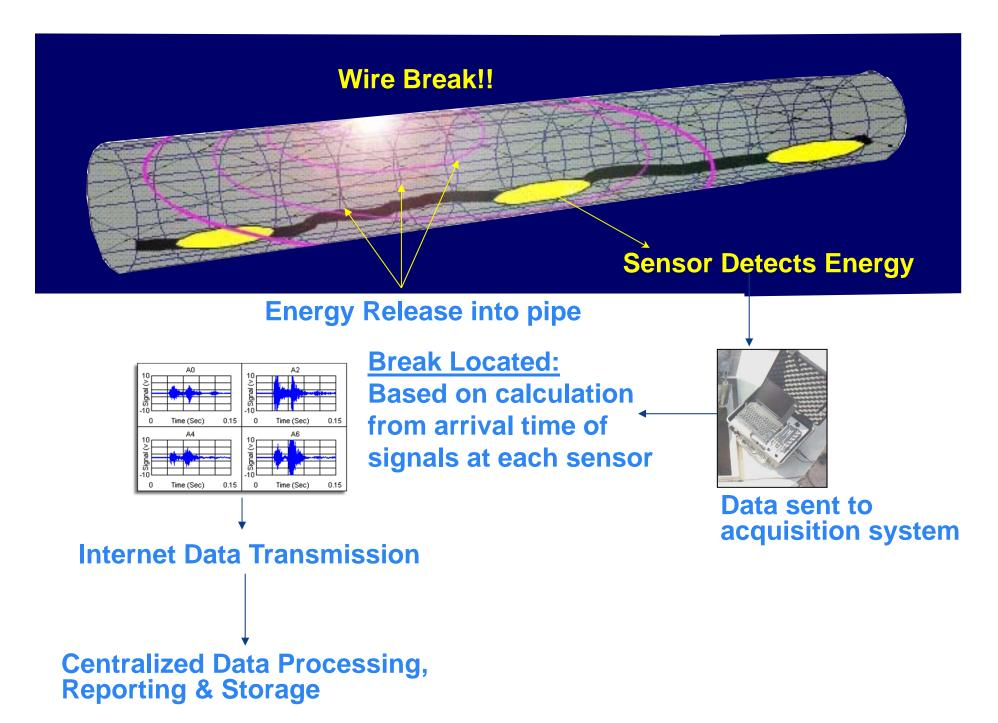
The arrays would be installed in one mile sections of the main for a 3-month period then moved to the next location.
