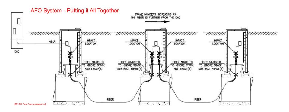
The acoustic fiber optic cable is able to "hear" and locate prestressing wire breaks in the pipeline as they occur.
