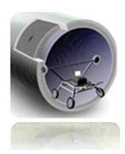
Phase II - A failure risk analysis is performed on each section of pipe that exhibits broken prestressing wires to determine the probability of failure.
