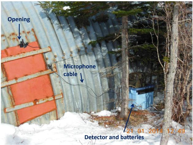
Figure 6. Setup of stationary detector at abandoned mine in Grand Mira, NS.
