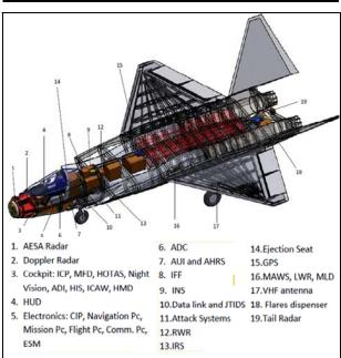
Fig. 17 Avionic installation.
