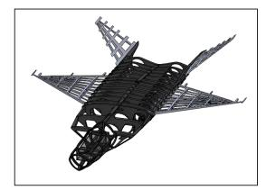
Fig. 16 Structures layout.
