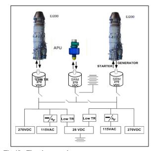
Fig. 18 Electric generation system.
