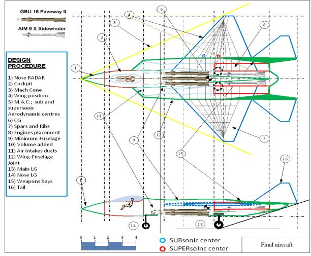
Fig. 14 Fighter layout definition procedure.
