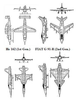
Northrop F 5 - A (3th Gen) Saab JAS 39 GRIPEN (4th Gen.) Fig. 6 Light fighter (of 1th to 4th generation).
