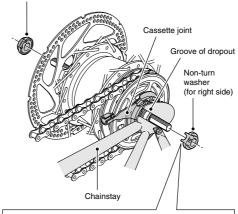
Use whichever non-turn washers match the shape of the dropouts. Different non-turn washers are used at the left and right sides.
