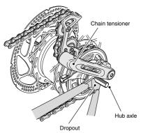
2. Place the non-turn washers onto the right side and left side of the hub axle. At this time, turn the cassette joint so that the projecting parts of the non-turn washers fit into the grooves of the dropouts. If this is done, the cassette joint can be installed so that it is almost parallel to the chainstay.
