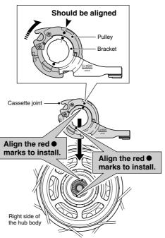
3. Secure the cassette joint to the hub with the cassette joint fixing ring. When installing the cassette joint fixing ring, align the yellow ● mark with the yellow ● mark on the cassette joint pulley, and then turn the cassette joint fixing ring 45° clockwise.
