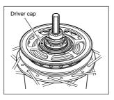
2. Turn the cassette joint pulley in the direction of the arrow in the illustration to align the red ● marks on the pulley and the bracket. With the cassette joint in this condition, install it so that the red ● mark on the cassette joint is aligned with the red
