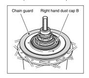
2. Install the CS-S500 sprocket to the driver on the right side of the hub body with the guard plate facing outward, and secure it in place with the snap ring.
