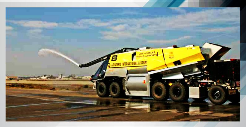
The Colet Jaguar series are the fastest and most advanced, all weather, fire-fighting crash vehicles in the world. The Colet Jaguar's active/reactive suspension system ensures greater vehicle mobility, performance, and safety. The Jaguar also features full crash cage protection and monocoque frame construction, elevating boom turret, forward-looking infrared night vision and GPS.
