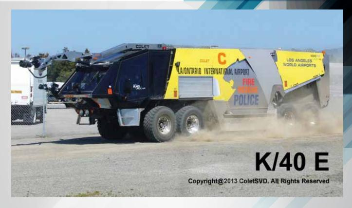
The COLET K/R40 Jaguar is the most powerful crash truck in the world. Some key features of the K/R40 are the PowerFlow Turret and Instatak firefighting systems. Together, they help make the K/R40 into an invaluable tool. The 1600HP engine pushes the K/R40 to 50 mph in less than 25 seconds, making it the fastest vehicle of its size in the world.
