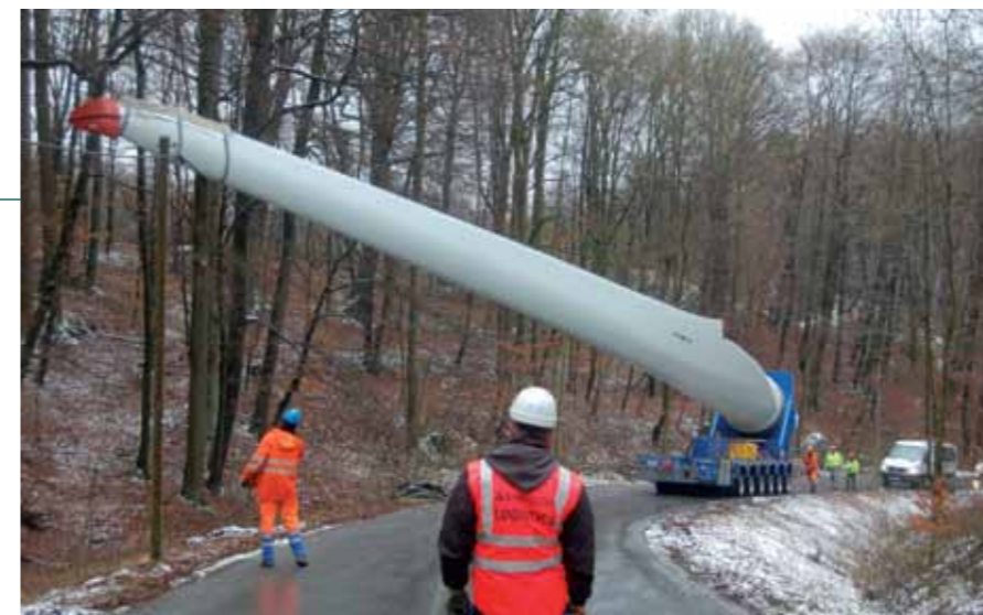
E-82 rotor blade on the alpine transport frame that was previously used successfully in the Alps.
