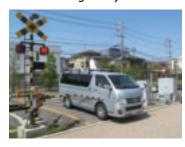
Omnidirectionally visible level crossing warning lights
