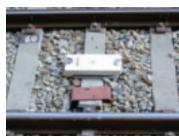
JR-West is installing ATS equipment for preventing accidents due to excessive speed.
