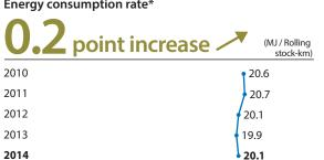
${\rm *The\ energy\ consumption\ rate\ is\ the\ amount\ of\ energy\ consumed\ per\ rolling\ stock-kilometer\ (MJ/Rolling\ stock-km)}$
