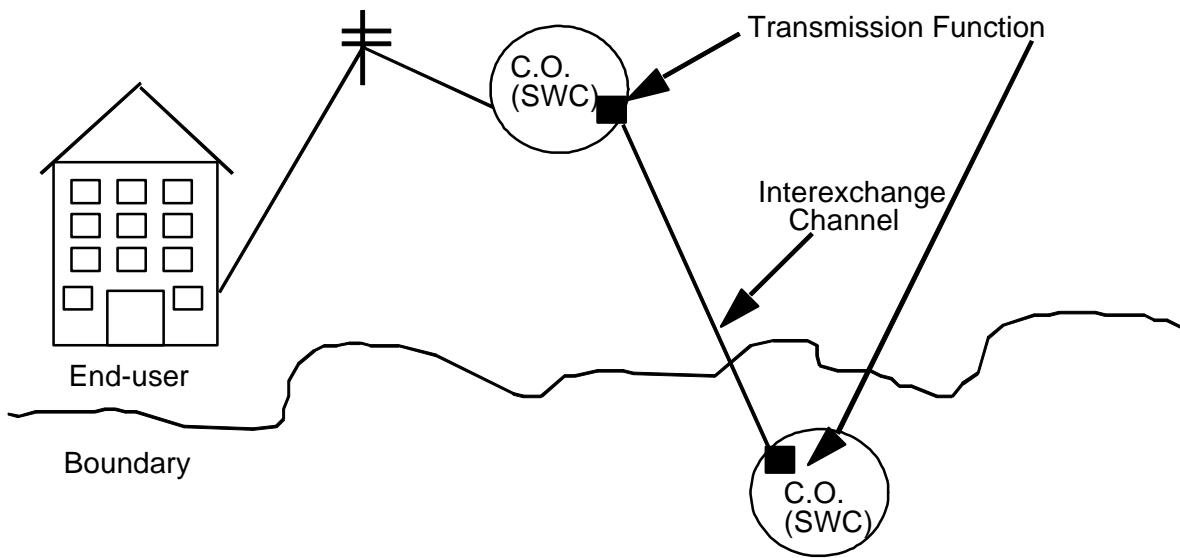
This diagram shows the end-user being served by a central office outside the boundary of the exchange area in which the end-user is located.
