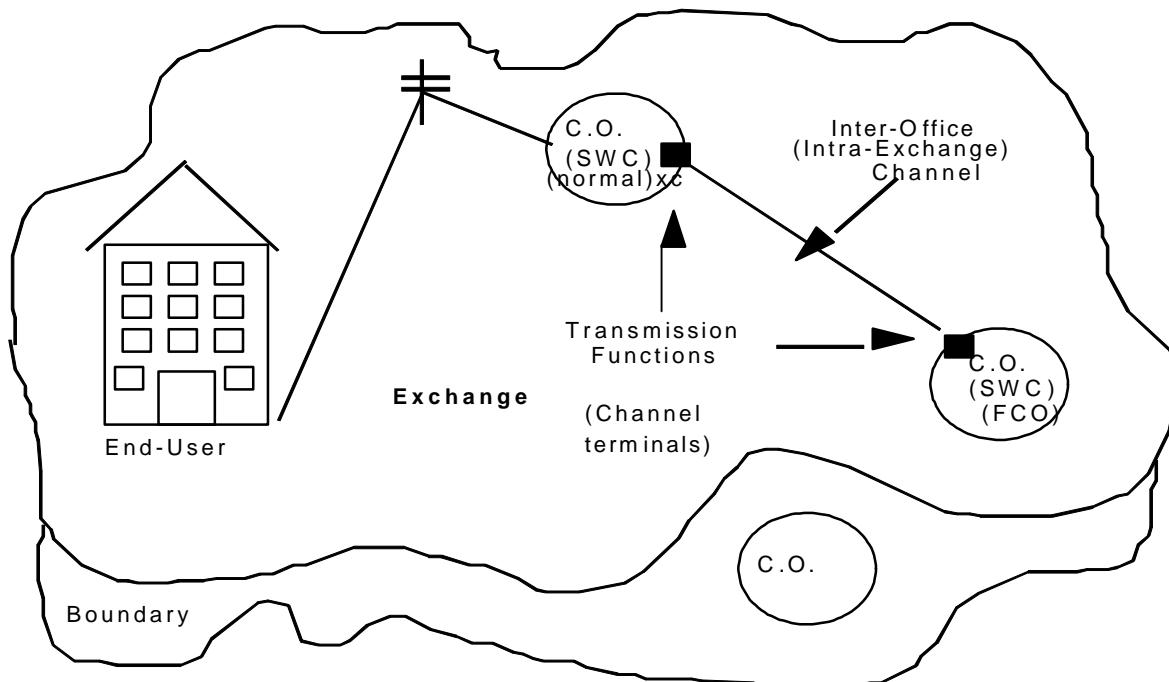
This diagram shows the end-user's location, with the line running to the pole and then to the normal central office that would serve the end-user. In this case, the end-user has requested a foreign central office (FCO) within the same exchange. Note that this is a multi-office exchange area. There is another central office located in a neighboring (contiguous) exchange area below the one in which the end-user is located.
