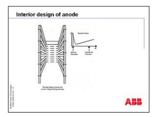
In real life it looked like this. The slide shows the final development step of an anode porcelain and intermediate electrodes. Six such anodes were connected in parallel to carry a line current of 2000 A.
