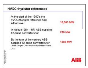
The developments in the 70's are impressive. The last mercury arc converters had a 12-pulse rating of about 500 MW, whereas the Itaipu thyristor 12-pulse converters have a rating of over 780 MW. And the size continued to increase to today's 1500 MW ratings for 12 pulse converters in the Chinese HVDC transmission schemes delivered by ABB.
