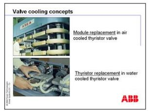
The first ASEA thyristor converters were air-cooled. Even though there was a lot of know-how in water-cooling for mercury arc valves, ASEA did not adopt this cooling method until later during the 70's. It was the German HVDC consortium that first demonstrated the efficiency of water-cooling in the Nelson River Project at the end of the 70's. This prompted ASEA following suite.
