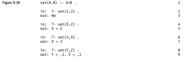
For free (unbound) variables, = constrains the value of the variable, and this binds it, as shown in lines 4 and 6. These values hold only for the duration of the search for solutions, not afterward. Line 9 shows that Y and Z have been bound together, both to the same don't-care result.
