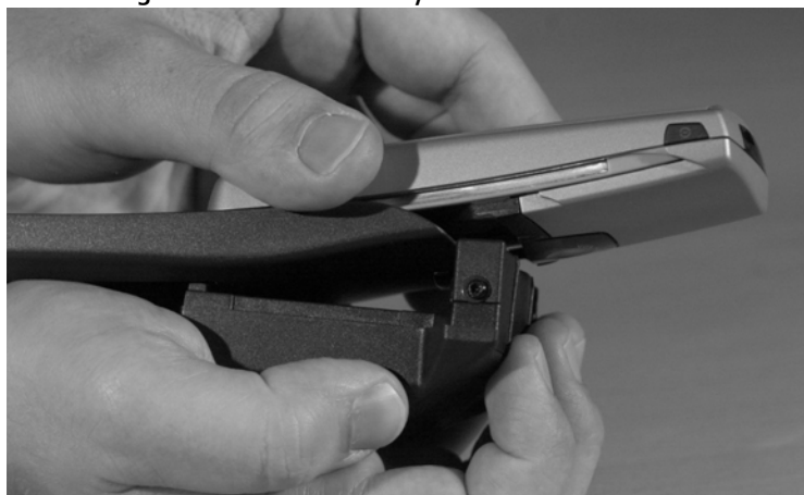
Figure 6: Connect battery connector to FLA-21:
