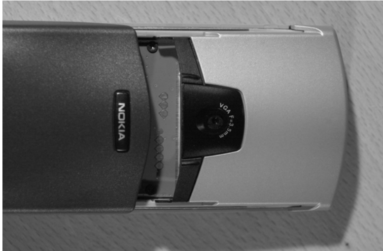
Figure 5: FBUS and MBUS pads visible when Phone has been opened to service position.
