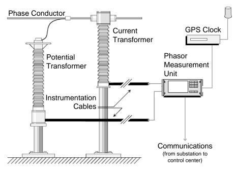
Figure 7. Example Synchrophasor System Installation within a Substation
