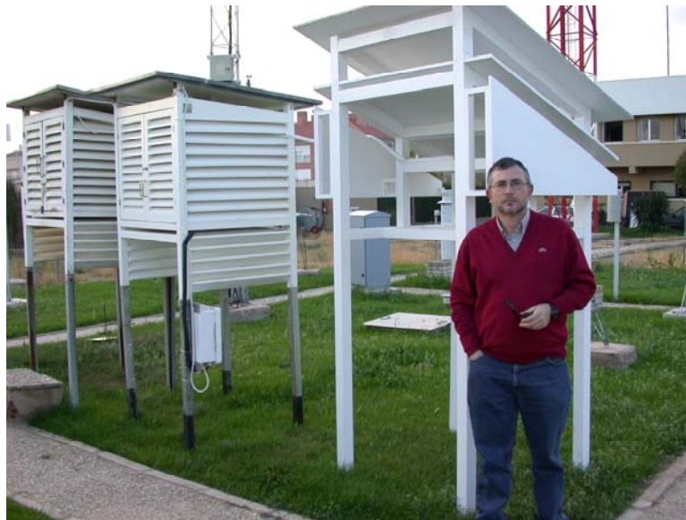
Figure 9: Experimental reproduction of historical measurements conditions. Parallel measurements are taken with identical sensors
