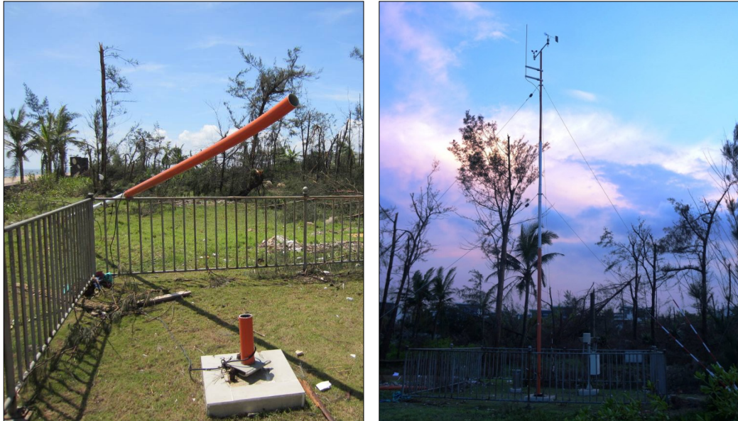
Fig. 2.5 left) On July 18, 2014, due to the Super Typhoon Rammasun, at the automatic station in Hailanyefeng residential district, Lingshan, Haikou, the stem cells were broken, and wind direction and speed sensors, wind cable, wind lever cables, lightning rod brackets were all damaged. Because of rainfall, collectors and pressure sensors failed. Right) On July 25, 2014, the image of the automatic station in Hailanyefeng residential district, Lingshan, Haikou after repair.
