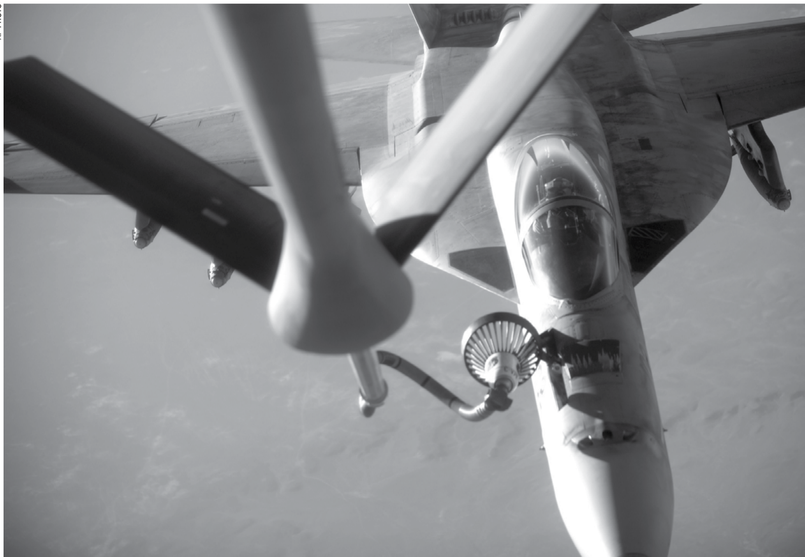
A U.S. Navy F-18E Super Hornet receives fuel from a KC-135 Stratotanker over northern Iraq after conducting airstrikes in Syria
