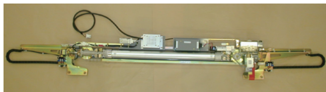
Fig.6 Door operating equipment
