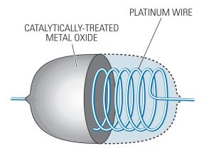
Fig. 4 A Catalytic Bead Sensor
