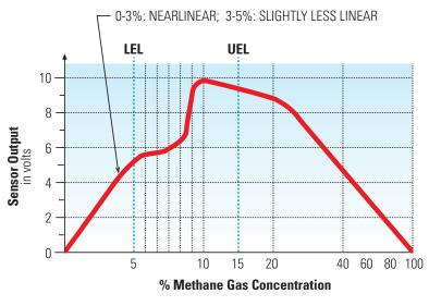
Fig. 5 Sensor Output vs. Gas Concentration
