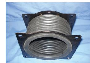
Traction motor blower duct
