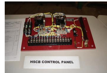
High speed circuit breaker control panel
