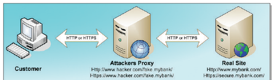
Figure 9: Man-in-the-middle attack structure
