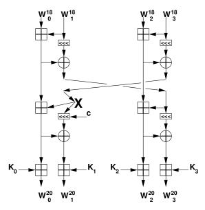
Figure 11: Simplified representation of rounds 19 and 20 of Threefish-256, including the key addition after round 20.
