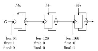
Figure 5: Hashing a three-block message using UBI mode.
