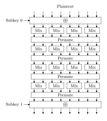
Figure 2: Four of the 72 rounds of the Threefish-512 block cipher.
