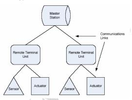
Figure 1: A typical 3-tiered approach to SCADA systems
