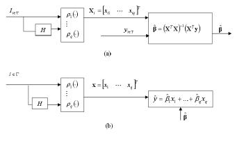
Fig. 3. Schematic description of (a) training and (b) testing.
