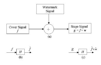
Fig. 1. Schematic descriptions of (a) watermarking or stegoing, (b) filtering an unmarked image, and (c) filtering a marked image.
