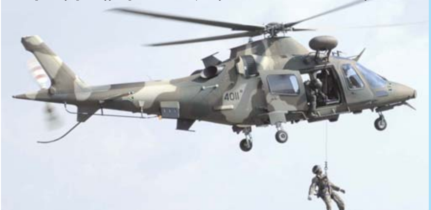
A109 light utility helicopter stretcher hoist demonstration.
