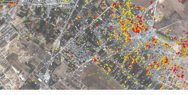
in some imagery specific conditions, damage to the facade is also apparent. All damage originating from small arms fire, heavy machine gun fire, and direct tank or artillery fire is generally not visible unless it results in some form of structural collapse. Given these limitations and the inherently conservative nature of satellite based damage assessments, the following classes of building damage were identified by UNOSAT:
