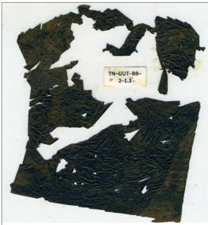
Figure 3. Sample of starch-based biodegradable plastic mulch (BioAgri) recovered after six months burial in the field at Knoxville. Photo J. Moore-Kucera.
