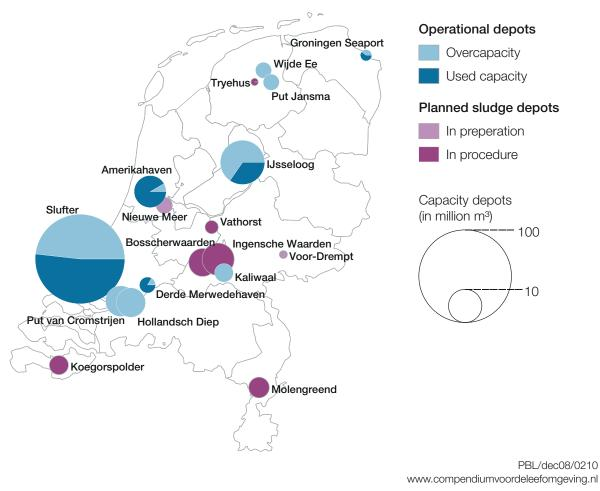
Figure 3: Depots for contaminated dredged material in the Netherlands.<sup>166</sup>
