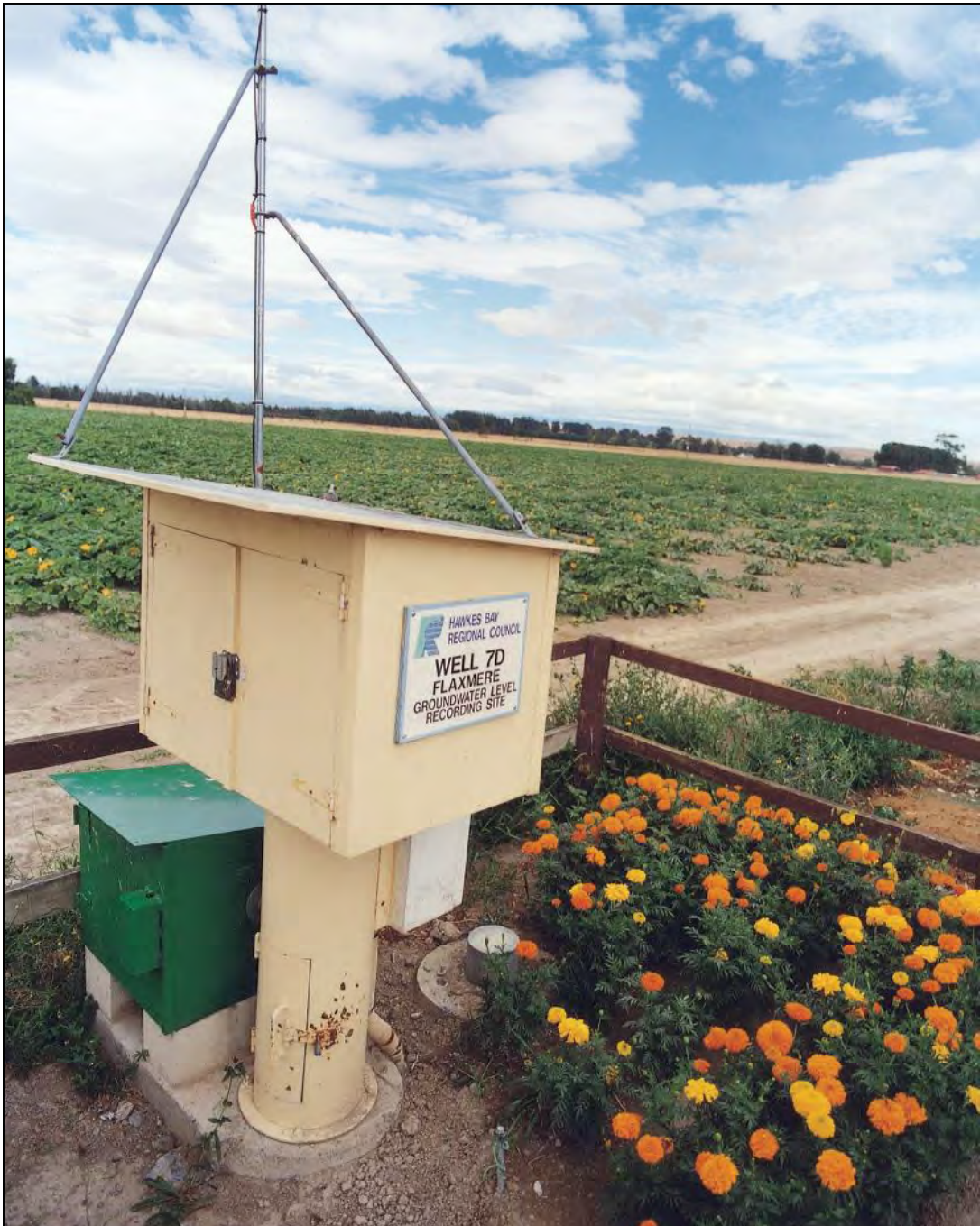
Figure 6.18: Well 7D (well no. 3737), Flaxmere showing housing for a continuous water level recorder. (photo: Lloyd Homer, IGNS CN 34 51)
