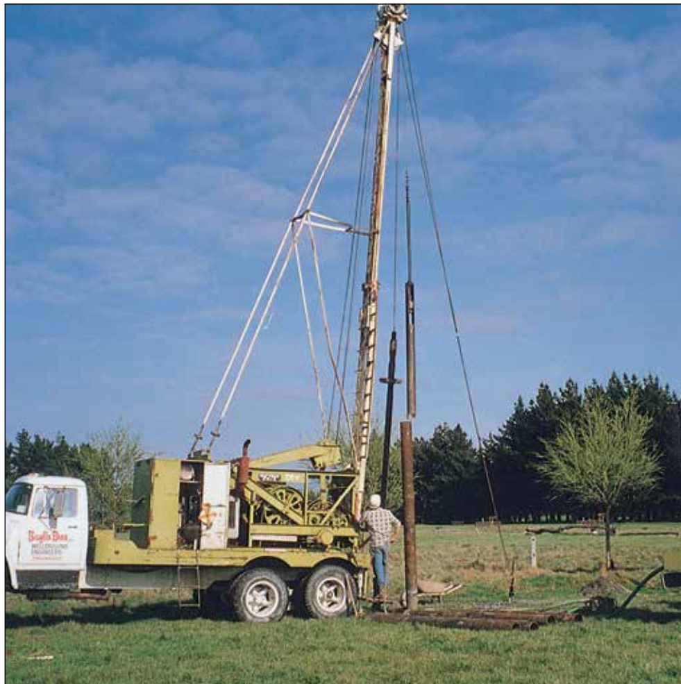
Figure 4.23: Baylis Brothers Erie 22W Cable Tool rig drilling Flaxmere testbore, September 1991. (photo: Len Brown, IGNS).
