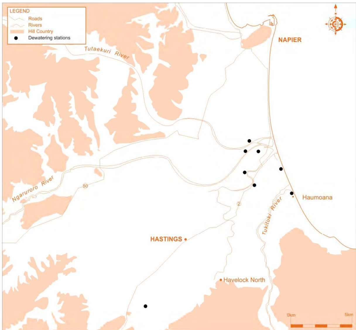
Figure 6.12: Coastal and inland shallow groundwater pumping (dewatering) stations.
