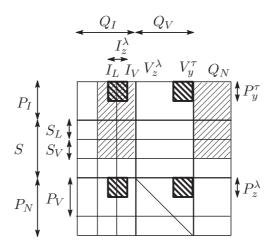
Figure 7: The coefficient matrix  $\tilde{A}(s)$  of MNA equations.
