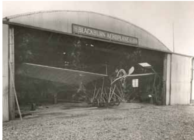
1911 Blackburn Mercury III (60hp Renault), wingspan 32' 0", Six aircraft built.
