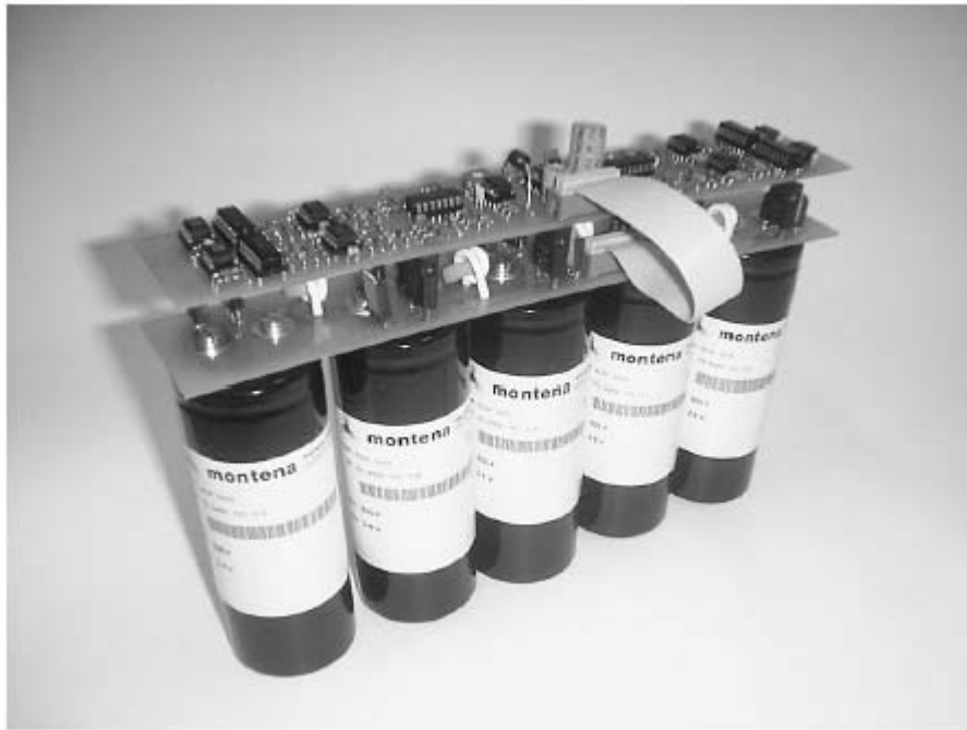
Figure 6.3 – A series connection of EDLCs including active voltage balancing [61].
