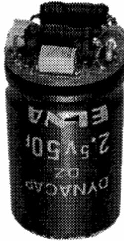
Figure 5.12 – An integrated supercapacitor and DC converter [55].
