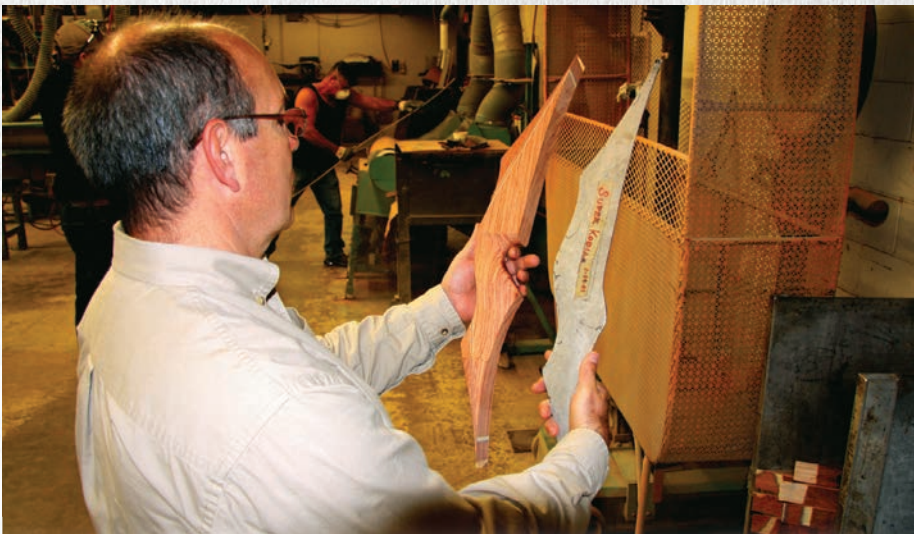
Bear Archery Products Operations Manager Neil Byce III compares a Super Kodiak bubinga handle section to the template used to assure risers remain within specs during production. The long tapers at each end assure a smooth transition into the recurve's limbs.
