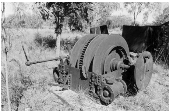
The dry climate of Croydon has preserved this little cast iron winding plant
