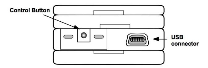
The connector is the micro-USB connector that allows the Sun SPOT unit to be connected to a host workstation.
