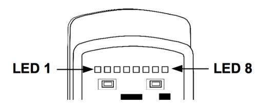
Each LED has a red, a green, and a blue emitter as part of the LED. Each individual color can have an intensity from 0 to 255, with 0 being off and 255 being as bright as possible.
