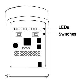
The LEDs have red, blue, and green components. The switches and LEDs have no pre-defined purpose and are under Java program control.
