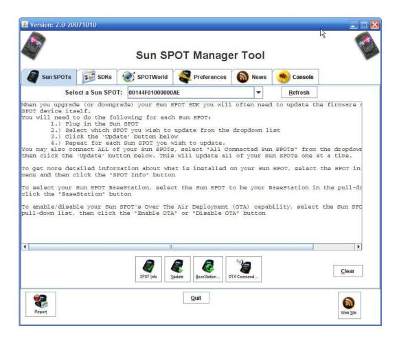
The menu above the console area is labeled "Select a Sun SPOT" and the pull-down menu lists all the Sun SPOTs that are connected by USB cables to the host workstation. Each Sun SPOT is listed by its IEEE network number. The first eight digits of this number are always 0014.4F01. The last eight digits are written on a sticker visible through the plastic surrounding the radio antenna fin on the Sun SPOT.
