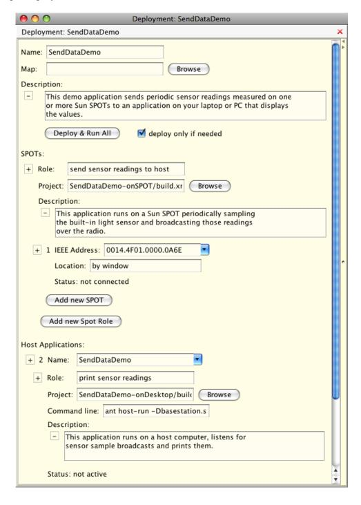
The deployment information is in three main sections. First is some information about the deployment as a whole. This includes the deployment name, an optional image file to be used as a map of the
