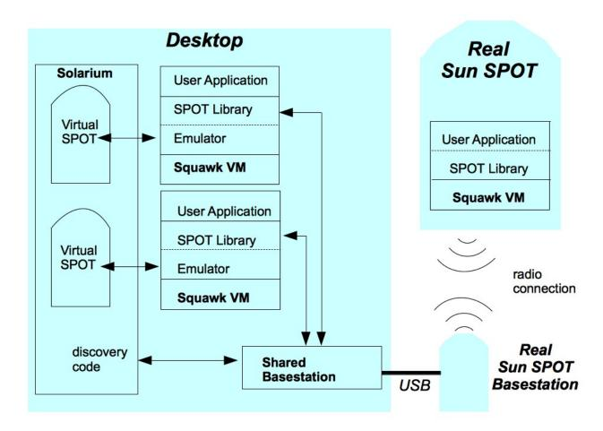
Each virtual SPOT has its own Squawk VM running in a separate process on the host computer. Each Squawk VM contains a complete host-side radio stack as part of the SPOT library, which allows the SPOT application to communicate with other SPOT applications running on the host computer, such as other virtual SPOTs, using sockets or real SPOTs via radio if a shared basestation is running.
