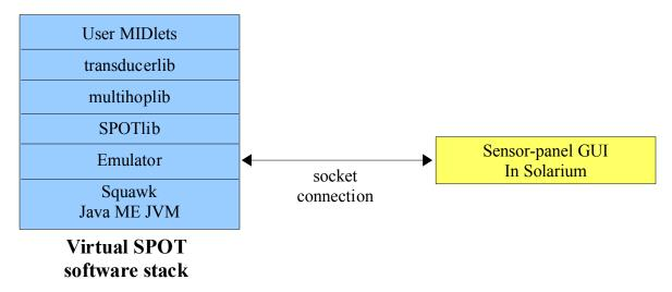
Each virtual SPOT has its own Squawk VM running in a separate process on the host computer. Each Squawk VM contains a complete host-side radio stack as part of the SPOT library, which allows the SPOT application to communicate with other SPOT applications running on the host computer, such as other virtual SPOTs, using sockets or real SPOTs via radio if a shared basestation is running.
