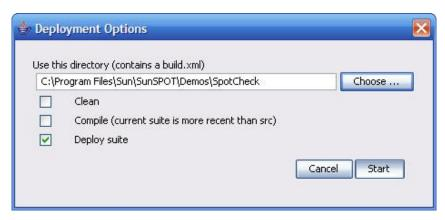
By default, the project directory will be cleaned, all source code will be recompiled and the resulting suite will be installed on the SPOT. The clean and compile steps may be skipped by unchecking the appropriate boxes. This might make sense, for example, if the application suite was created recently and the same suite is being deployed on multiple SPOTs.
