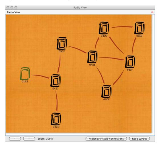
When the Radio View window is first opened, Solarium sends commands to each known SPOT asking it to discover its neighbors. The red lines show which SPOTs that can exchange radio packets. After all the SPOTs have replied a graphing algorithm is used to create the best layout that shows the radio topology. The Radio View has no knowledge of where the SPOTs are located physically, so the layout algorithm can only try to minimize the number of connections that cross each other.
