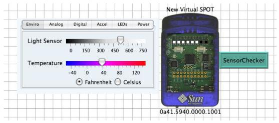
read from one of the SPOT's sensors. When it is started the light sensor reading is displayed in white. To change the light sensor value use the **Display sensor panel** command to bring up the sensor panel. On the leftmost *Enviro* tab are two sliders for controlling the value the SPOT will read for the light sensor and for the internal thermometer. As you move the light sensor slider left and right you will see the number of LEDs change appropriately.
