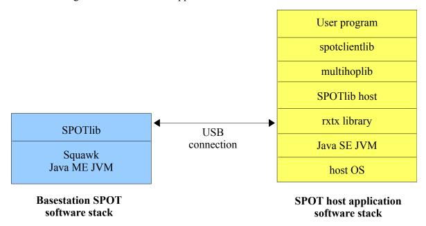
Again at the top is the user-written host SPOT application, which is just a regular Java SE program. It can do everything a regular Java application can do: file I/O, display Swing GUI's, etc. It can also send and receive radio messages with free-range SPOTs if a basestation is connected to the host computer.
