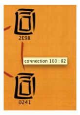
Link Quality is uniquely determined by the CORR value: CORR is a correlation measure provided directly by the radio part. Link Quality values range from 100% (the best, corresponding to a CORR value greater than 100) to 0% (the worst, which means the CORR value is less than 50).
