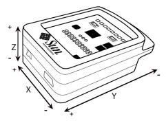
In the figure above, the plus (+) on the end of an axis indicates that when the device's acceleration vector increases in that direction, the associated accelerometer readings grow larger.
