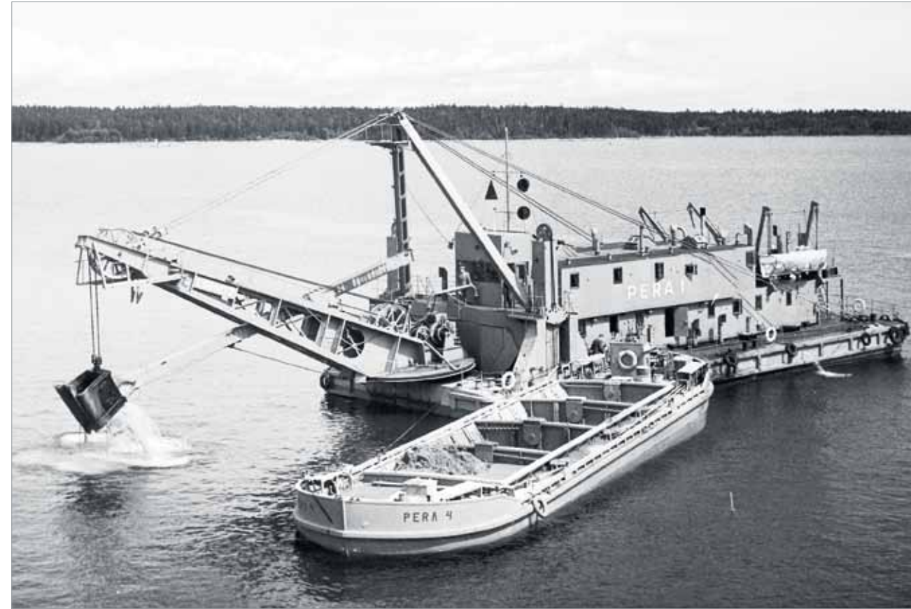
In Finland, the dredger Pera I was acquired in 1957 with funding from the World Bank. The dredger deepened ship channels to serve marine transport of imports and exports.
