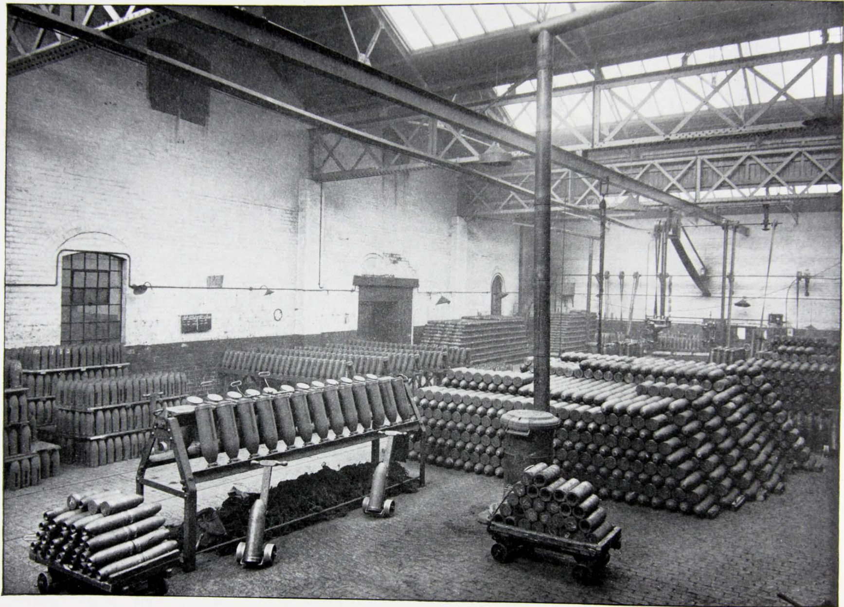
BELGRAVE GATE.—Main Shop, showing painting racks and shells ready for despatch to filling factories.
