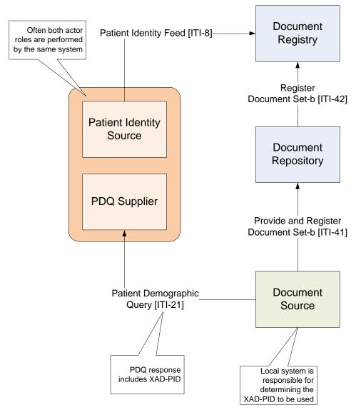
Figure 3.1-1 Decentralized XAD-PID Matching using PDQ
