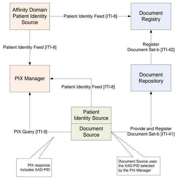
Figure 3.2-1 Centralized XAD-PID Matching
