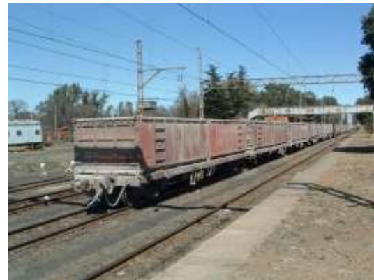
Intermodal 6 m open-top containers with lime at Viljoensdrift station. (6.3)
